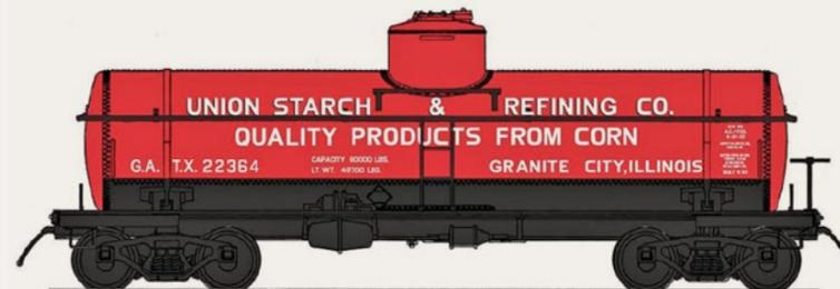
InterMountain plans to release another run of its 8,000 gallon ACF Type 27 tank car in February or March. In addition
