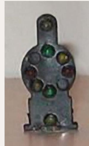
The **NJ International** ([njinternational.com](http://njinternational.com)) booth at the National Train Show displayed a wide range of signals including new O scale Union Switch & Signal type VA dwarf CPL (color positional lights) signals as used by the Baltimore & Ohio Railroad. The group includes a basic 8-light, 4-position dwarf and a similar signal with one marker (left). Visit the above website for complete details including pricing.
