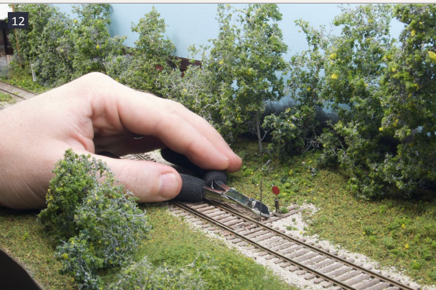
12: The excess wire is trimmed with the top of the throwbar using flush-cut pliers.
