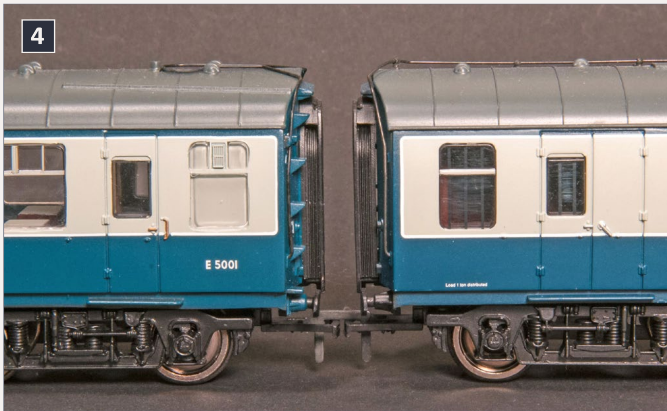
4: These Bachmann Branchline UK cars have a fixed diaphragm at each end that allows a gap to show in the corridor connections of passenger trains.
