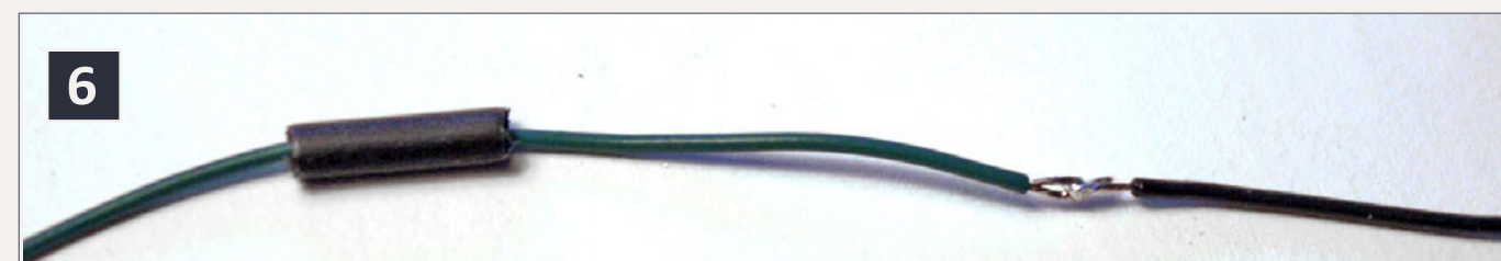
6: Soldered splice, ready for shrink tubing.
