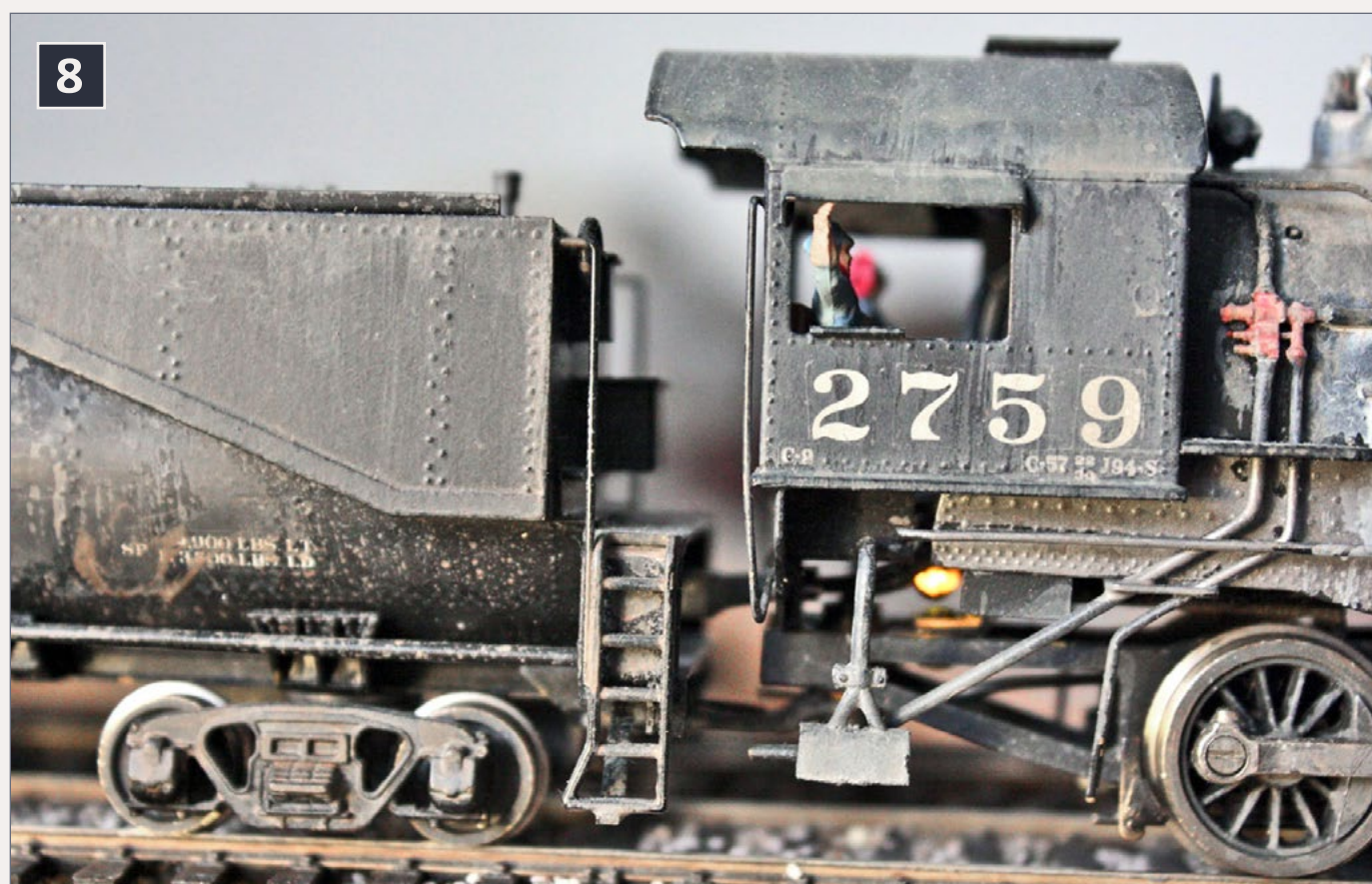
8: This shot shows the “Firebox Flicker” LED at rear of firebox, and the flat cable to the tender can be seen just to the left of it. Drawbar is down below it.
