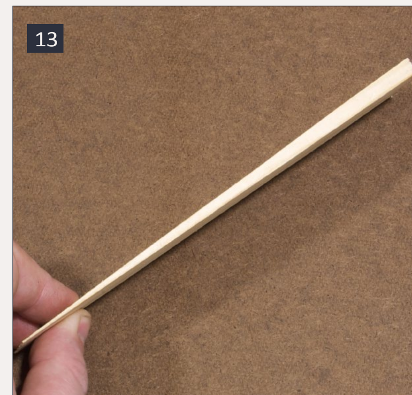
13: A contractor's wood shim provides the right amount of leverage to pull the wire down through the throwbar and sub-roadbed while being lightweight and simple to install.
