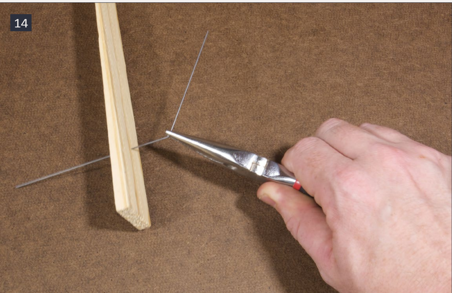
14: The piano wire is threaded through a hole drilled in the shim and bent along the bottom so gravity will pull both the shim and the wire down when unlocked.
