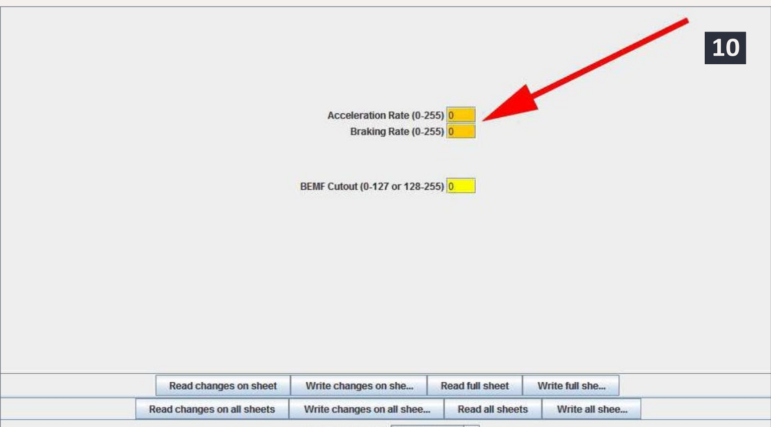
10: DecoderPro screen: Setting momentum in the MOTOR tab – This is for a TCS T1. You can see the BEMF cutoff settings in this tab, too.
