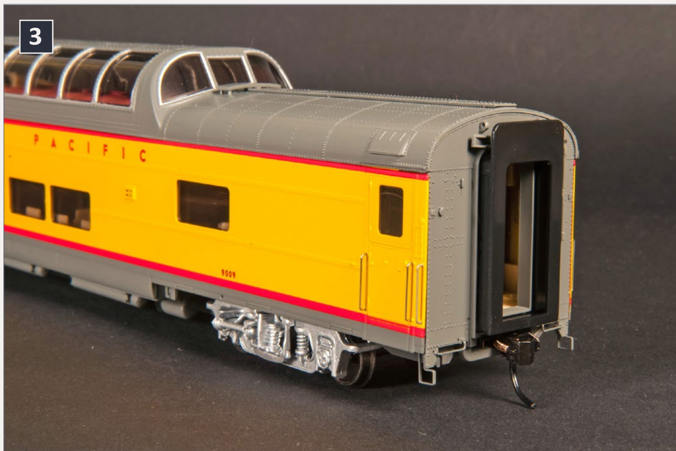
3: Walthers represents the diaphragms at the end of its new passenger cars with a springy, sliding housing to keep the gap between cars filled.
