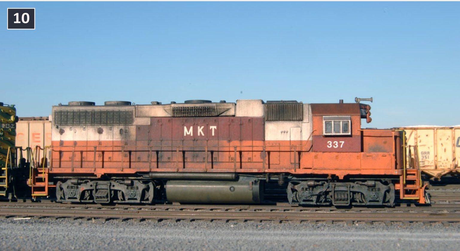
10: Modeled after an ex-ICG engine that the Katy bought in the mid-1980s, this Lifelike GP38-2 was factory decorated and patched by Scott to match the prototype. He changed details to make it an accurate GP38AC, and added a single chime air horn, air filters, MU hoses, air lines, and Sergeant couplers.
