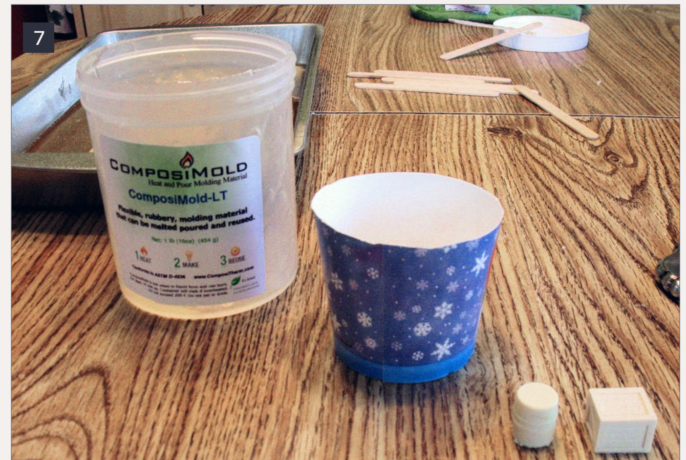
7. The mold box for an O scale barrel and crate consists of a cut-down paper cup.
