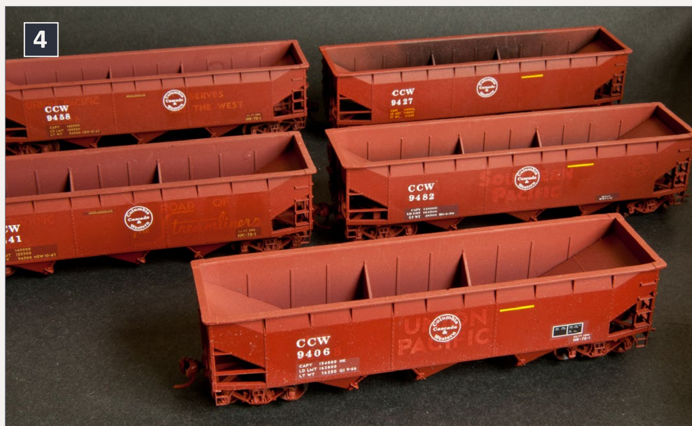
4: Accurail hopper cars painted using Krylon spray cans.
