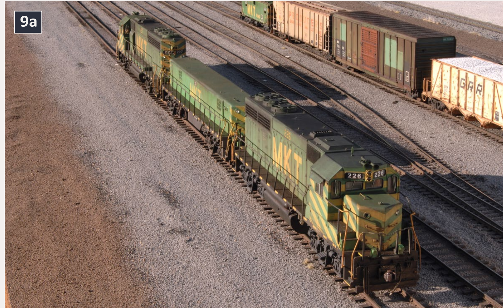
9a-9b: The MKT slug-mother set operates as a single unit and was never parted, except for heavy maintenance. Katy crews nicknamed the set "The Three Stooges."
