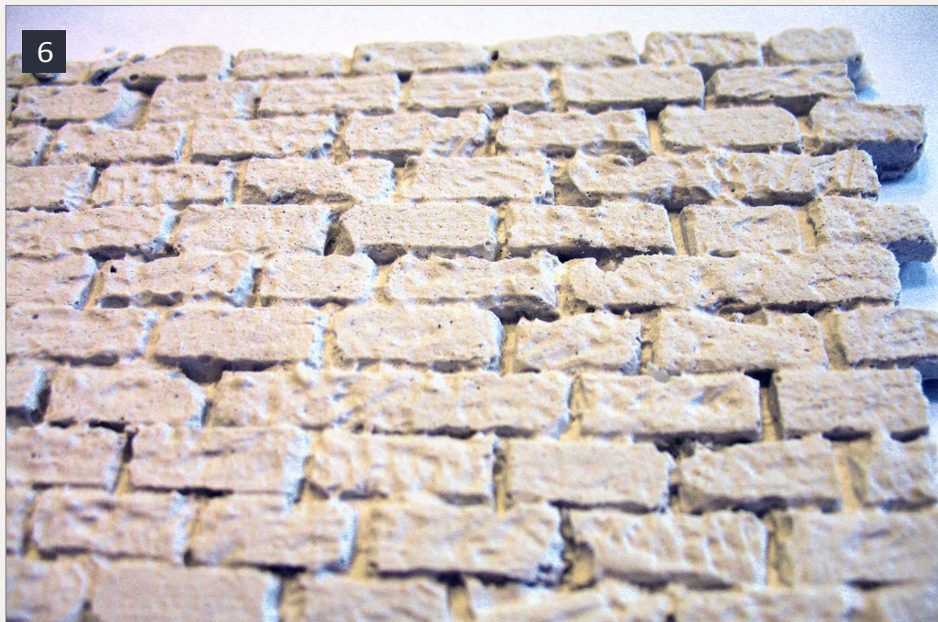
6. Completed plaster casting. The tiny bubbles seen are in the plaster pour, and not in the mold.
