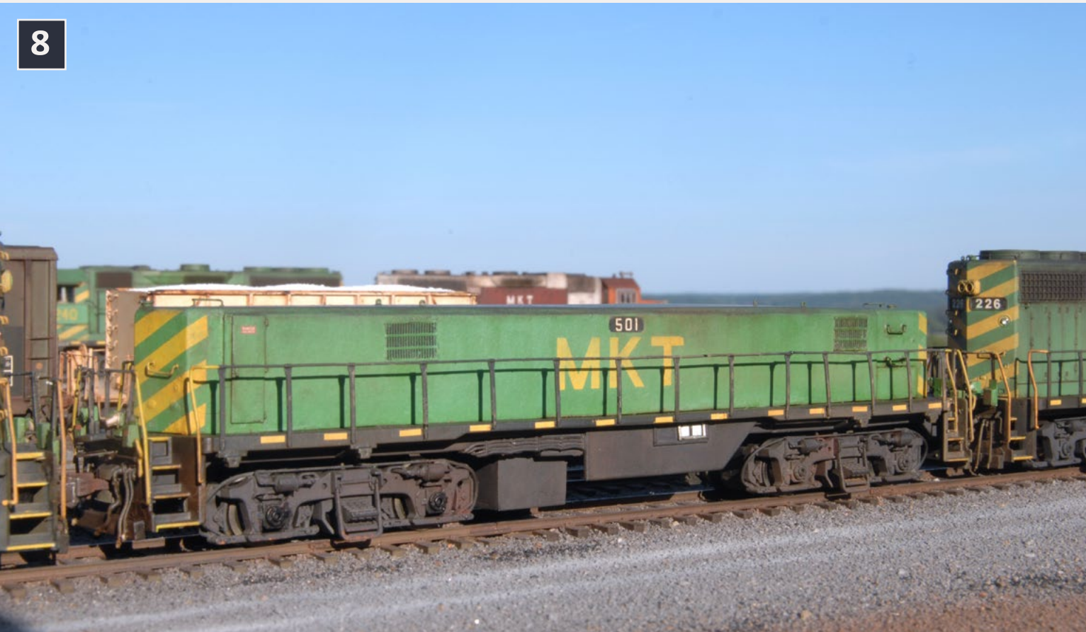
8: His custom-built slug uses an Atlas frame and trucks. The body is built from styrene and painted with Modelflex. Added details include MU cables, actuating hoses, sand lines, traction motor cables, and oil and pastel powder weathering.
