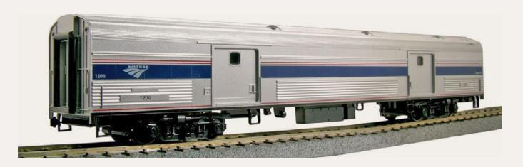
**Kato USA** (<u>katousa.com</u>) has added a baggage car to its lineup of Amtrak Superliner models. Features of the HO scale ready-torun model include prototypical exterior fluting and appropriate trucks with working bearing caps and shock absorber. Optional Kinematic tight-lock couplers are included. The late additions to the Superliner group will be available in two road numbers in Amtrak's phase IVb scheme. The final MSRP is estimated at \$85.00 to \$90.00 each.
