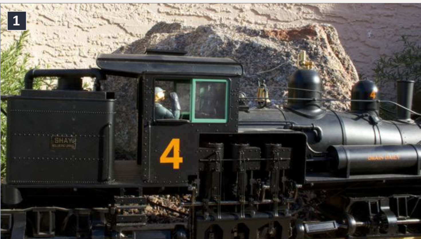
1: Loco with a short cab address of 4 – I run it as a long address on NCE by programming it as a long address and selecting it as 04.
