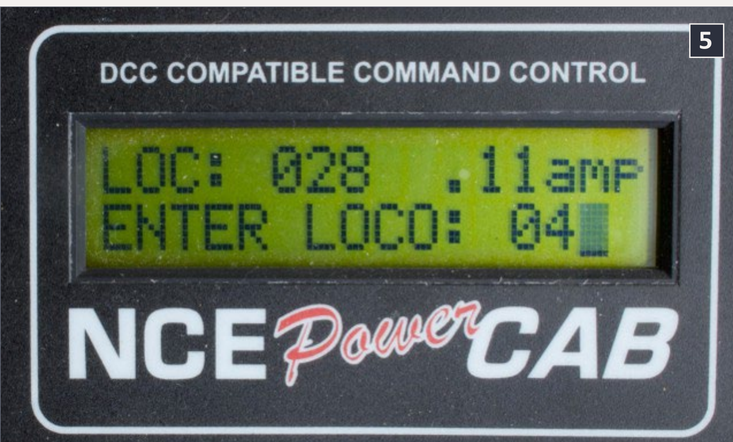
5: Programming the loco from figure 1 into an NCE Power-Cab with a long address of 04.
