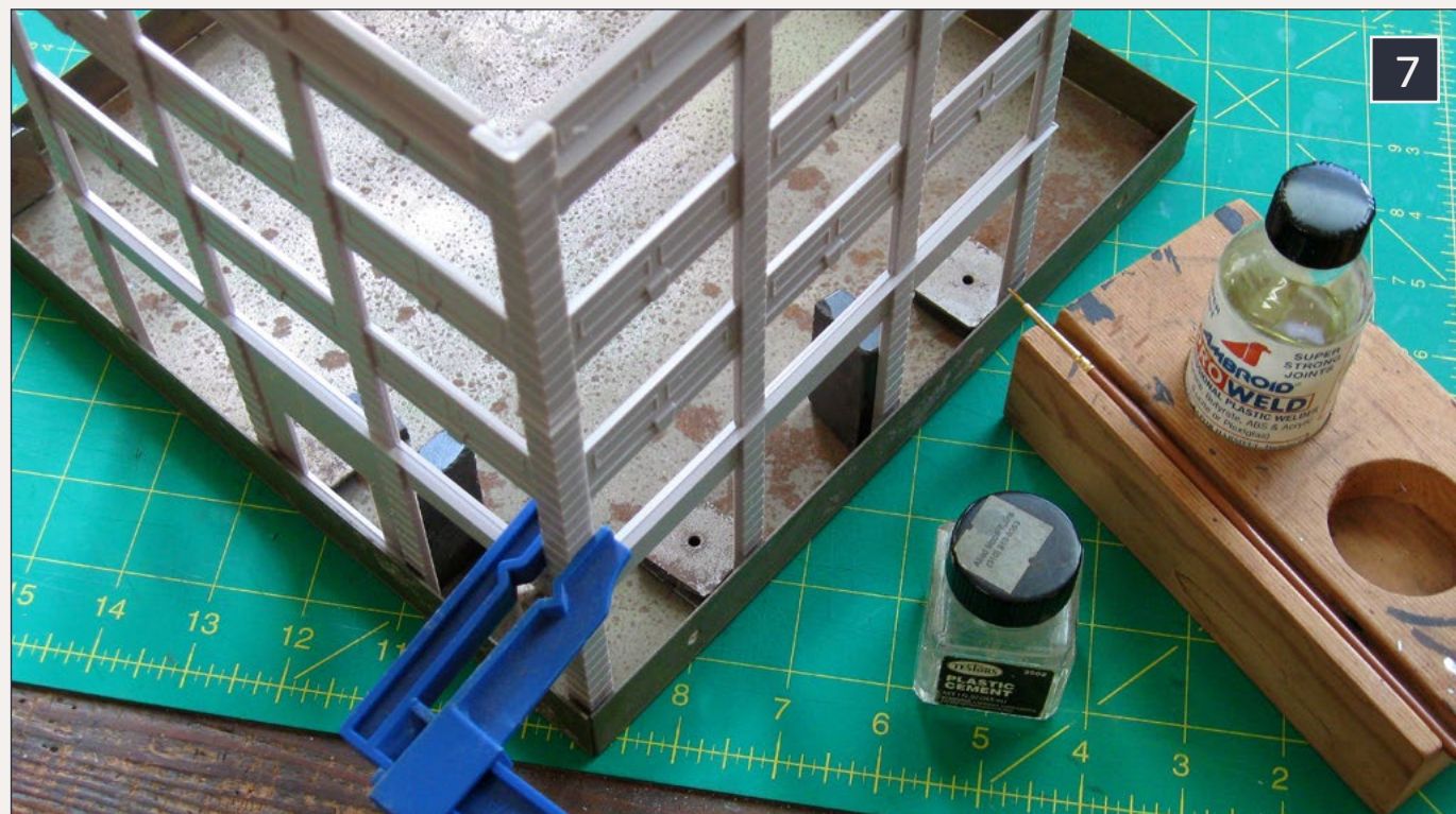
7: My trusty (and rusty) old magnetic jig keeps walls square as cement dries.
