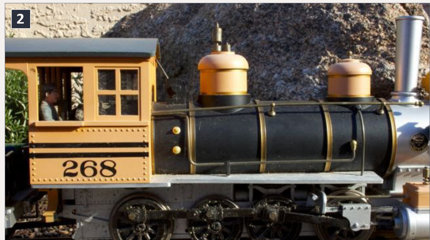
2: Loco with cab address of 268 – this will be a long address on any system, even though it has only 3 digits.
