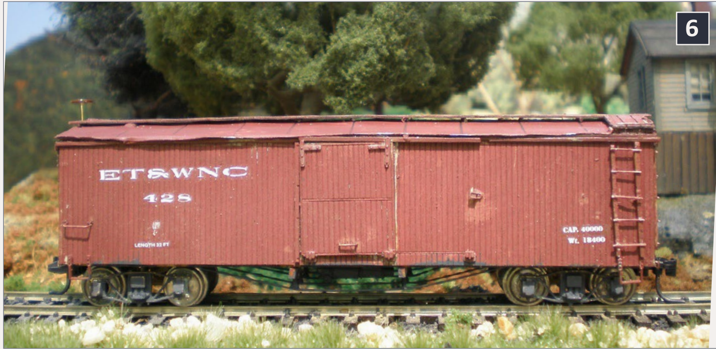
6: Tweetsie box car built from Train and Trooper laser kit. The trucks are the proper ones for the car (McCord archbars) and this is typical of the 32' cars operated by Tweetsie.
