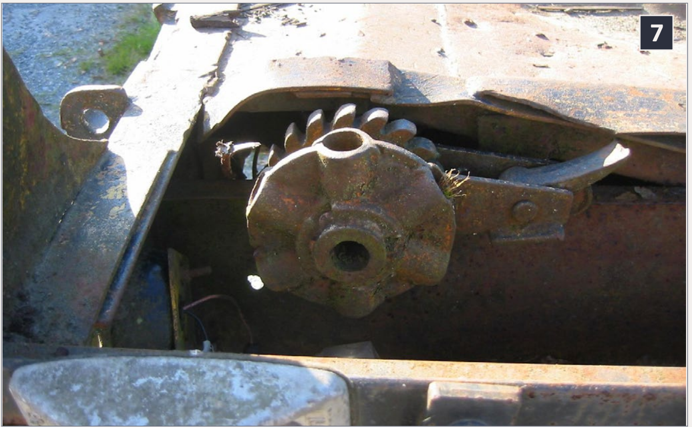
7: Here is detail of the ratchet system that is used to tie down the autos during transport.
