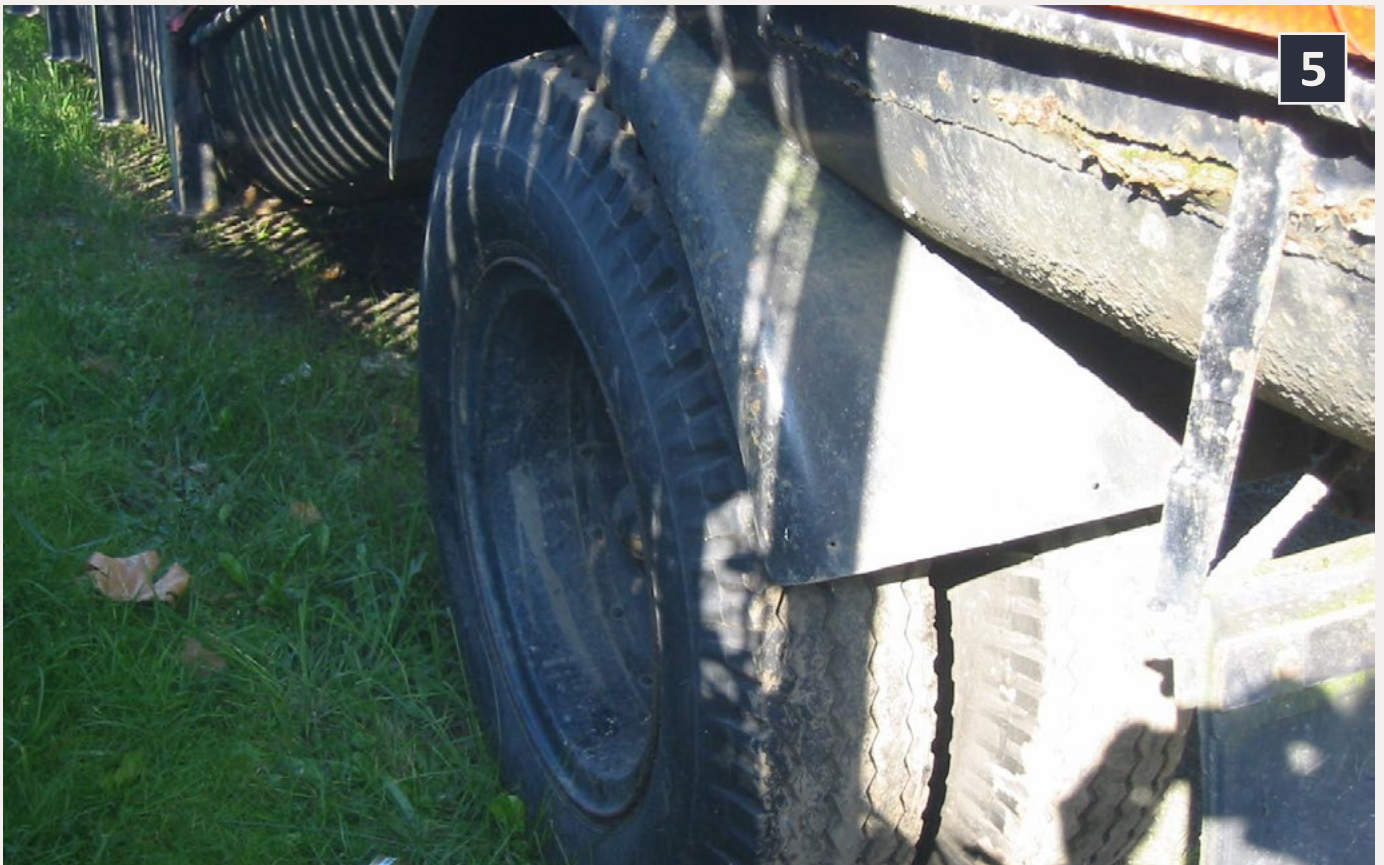
5: Details of the rear axle. Notice the fender over the wheels. The mud flaps are located farther back.
