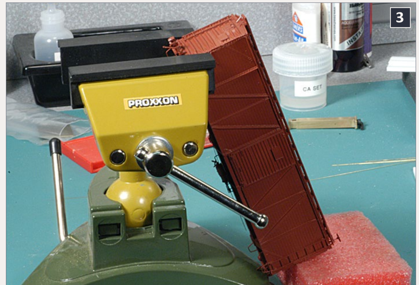
3: I've turned the vise (and boxcar) 90° to provide a better view of the setup. The bottom end of the car rests on a scrap of dense foam. This raises the car enough so the other end rests between the jaws. Note that only a portion of the bottom of the end of the car rests on the red foam. In order to avoid the need wait while the decals dry enough to handle the car, I first decal one side of the car and then one end. I then swap the car end-for-end and decal the second end. By then the decals on the first side have dried, and I can decal the second side.
