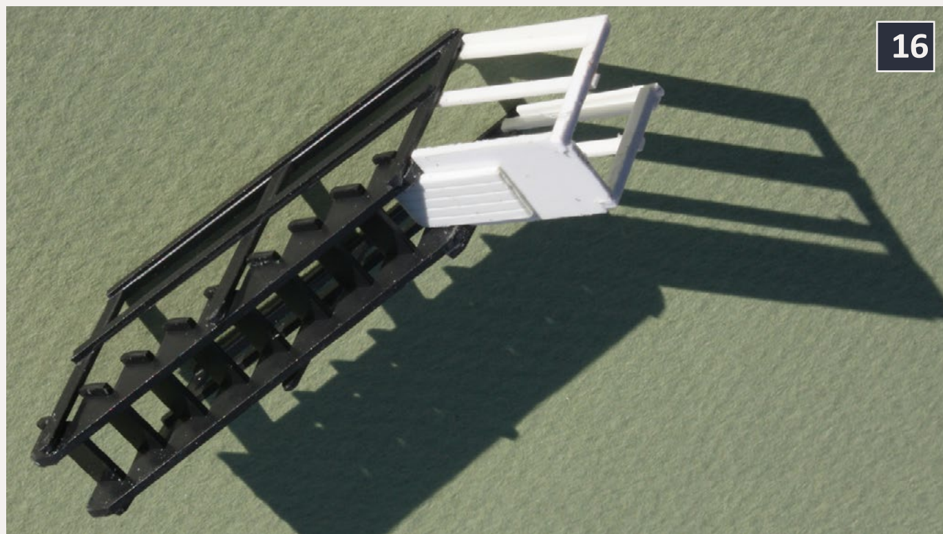
16: This view from beneath the stairway assembly may clarify the construction of the horizontal walkway, and clearly shows the splice plate attaching the two parts.
