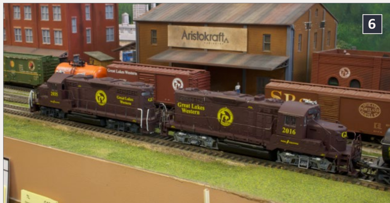
6: Consisted locos on the PCMRC layout – consistent loco and decoder design and attention to detail allow them to run together with BEMF activated.
