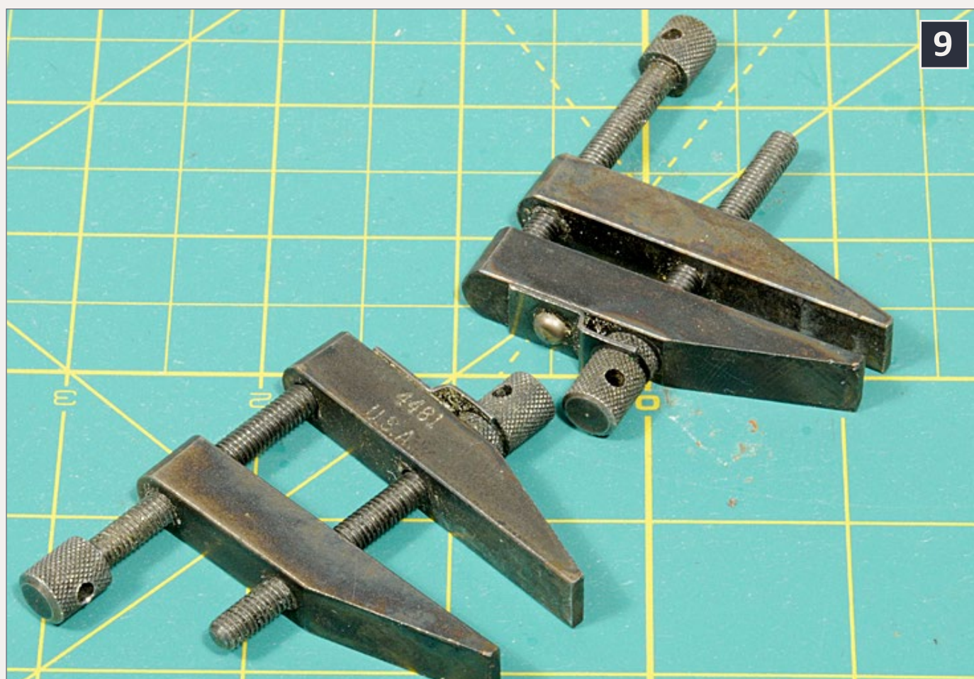
9: The jaws on these machinist clamps are tightened by turning one screw in while turning the other screw out.
