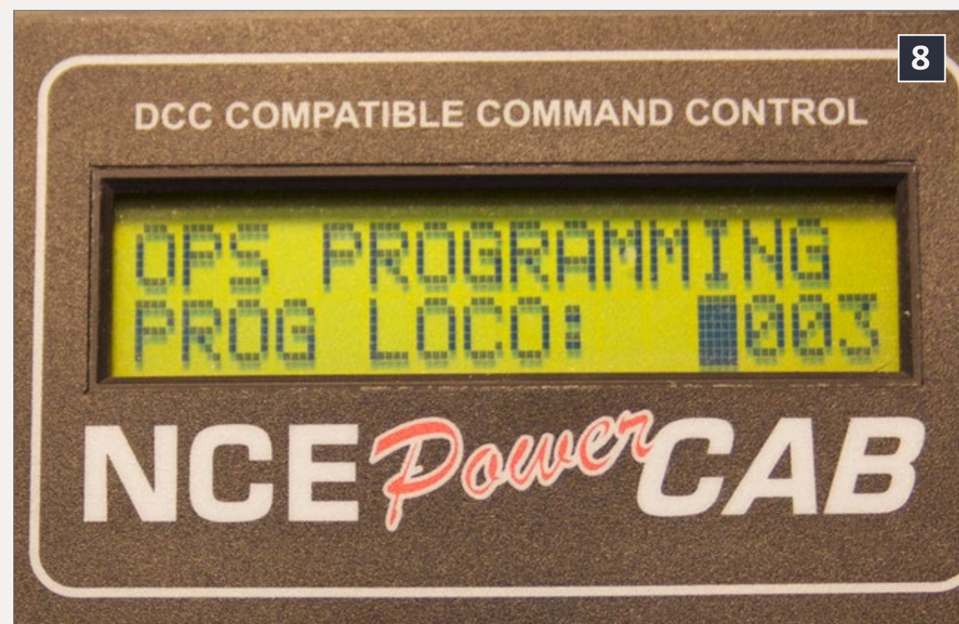
8: PowerCab POM screen asking for locomotive address.
