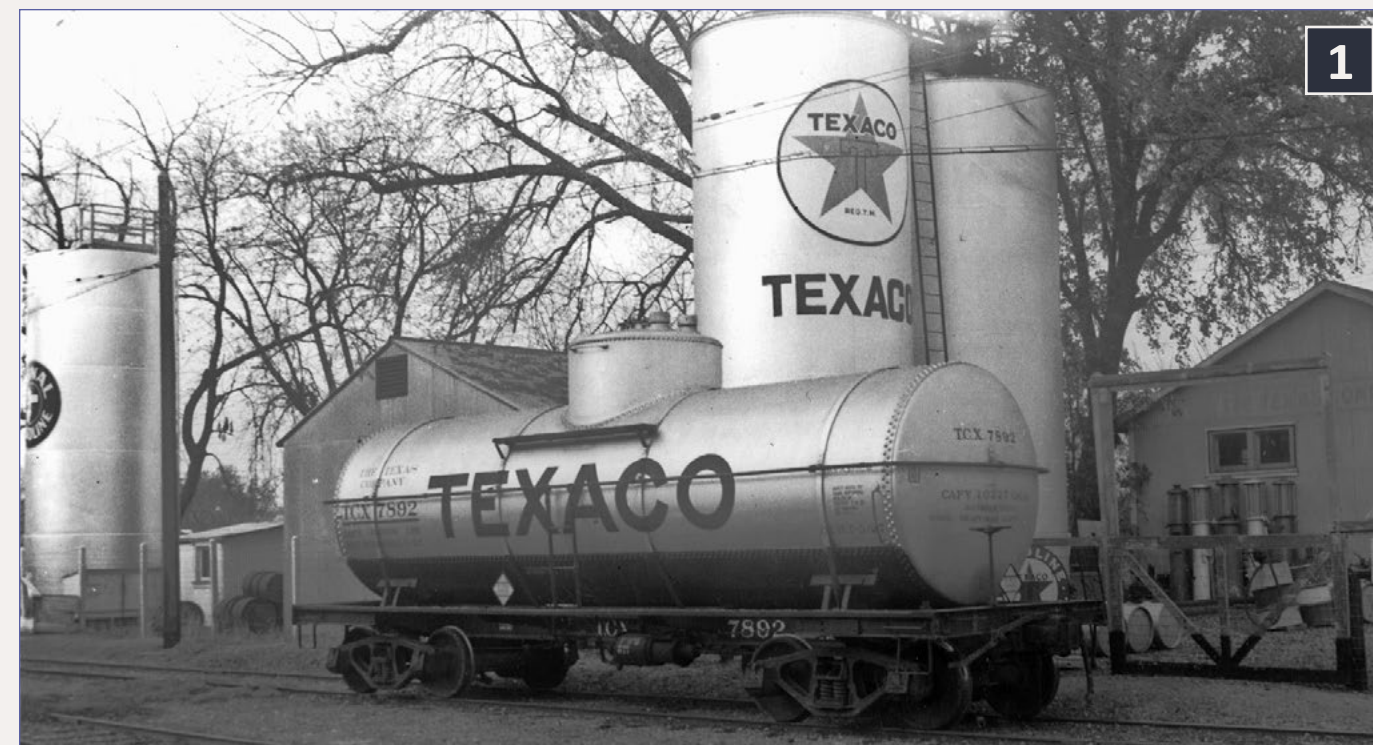
1: A Texaco bulk oil dealer, in Woodland, California, December 17, 1939. The siding is part of the Sacramento Northern (by this time a property of the Western Pacific). This silver tank car is a relatively rare car with such a paint scheme, assigned to deliver consumer products and thus given a brighter paint scheme. Note also the adjoining dealership, with its Signal Gasoline tank logo – Wilbur C. Whittaker photo.
