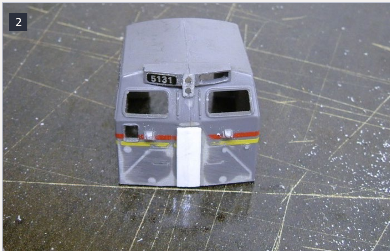
2. The new smaller cab with new door. The cut is barely visible.
