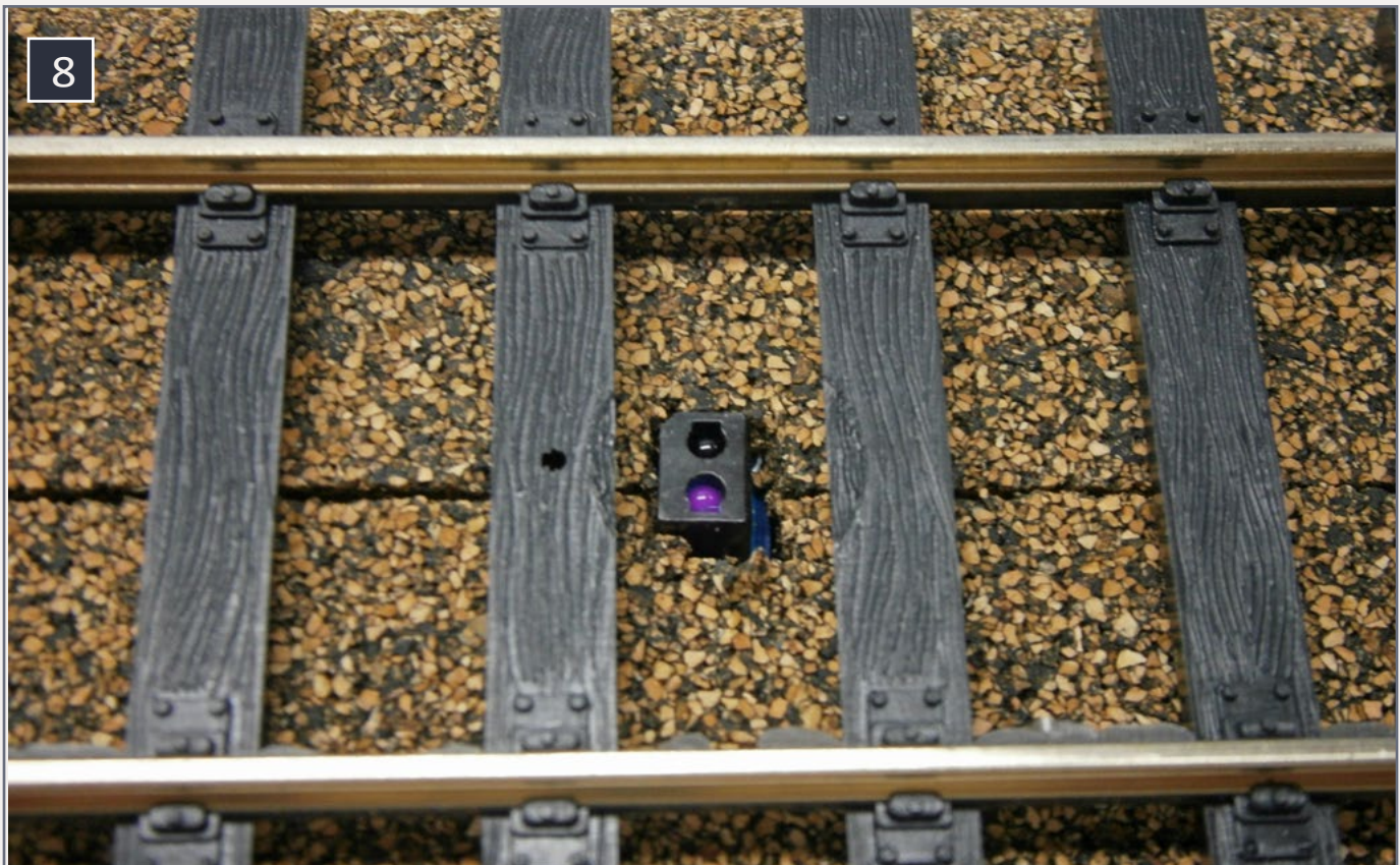
8. The sensor mounted below the track.
