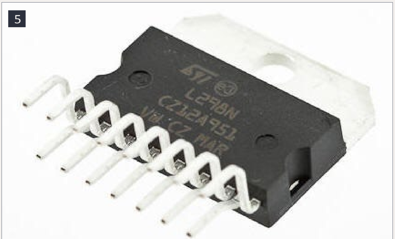
5. The L298N H-bridge, the “brawn” of the PICAXE controller.
