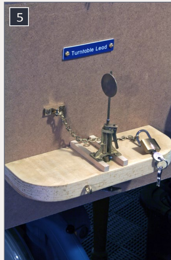
5. The same switch stand unlocked and lined for the diverging route. The target is now perpendicular to the fascia.
