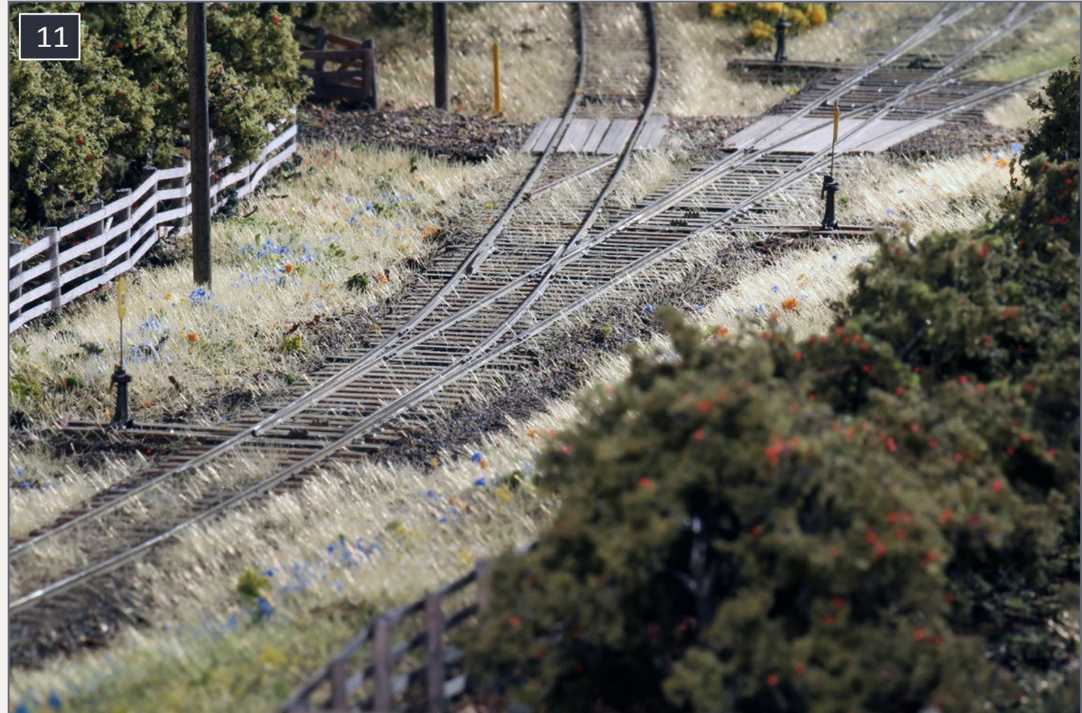
11. To help operators confirm that the turnouts have been thrown, S scale switch stands with swivelling targets are mounted to the head ties of each switch.
