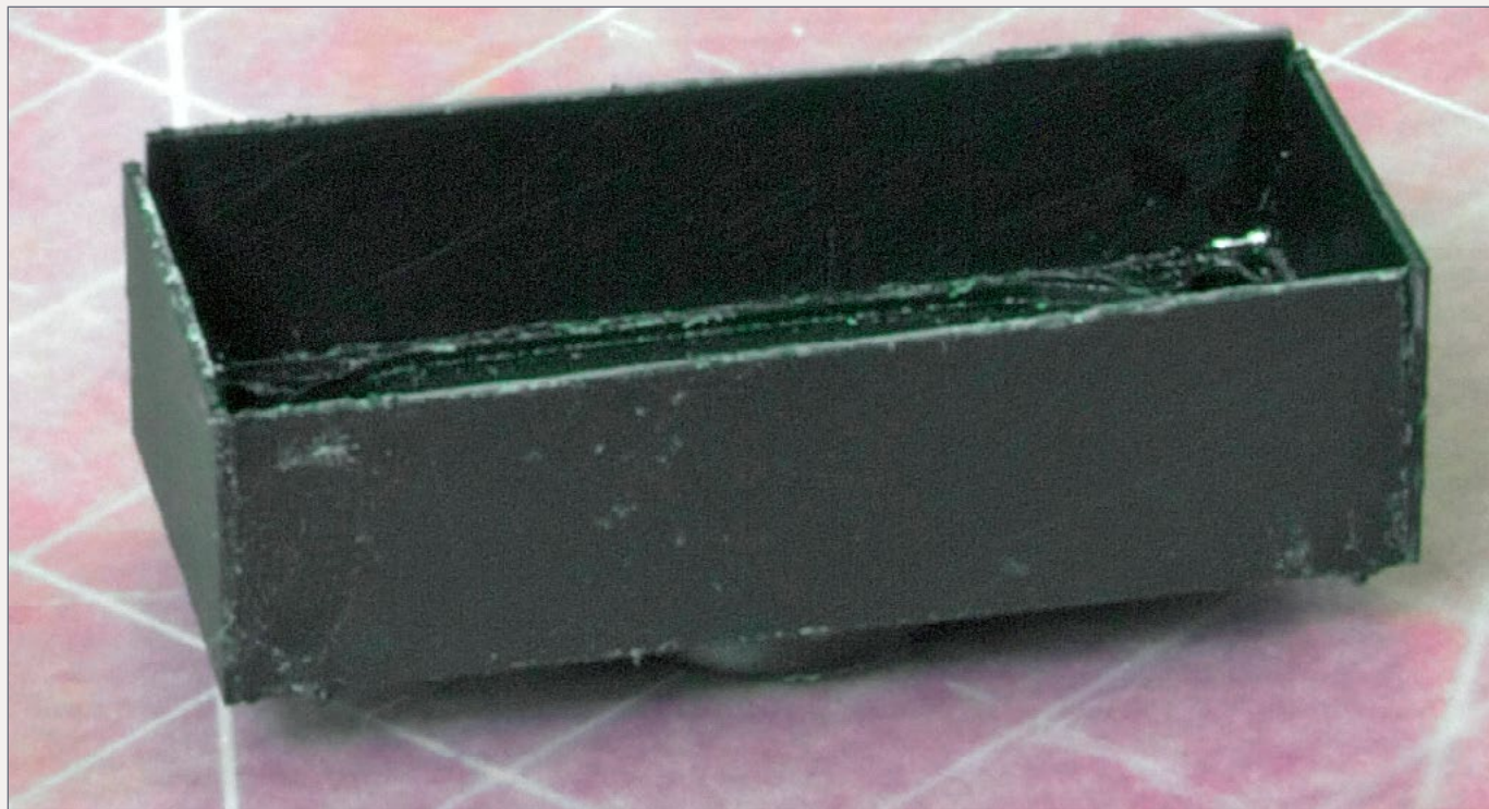
5. Speaker enclosure under construction - ready for last side to be added.
