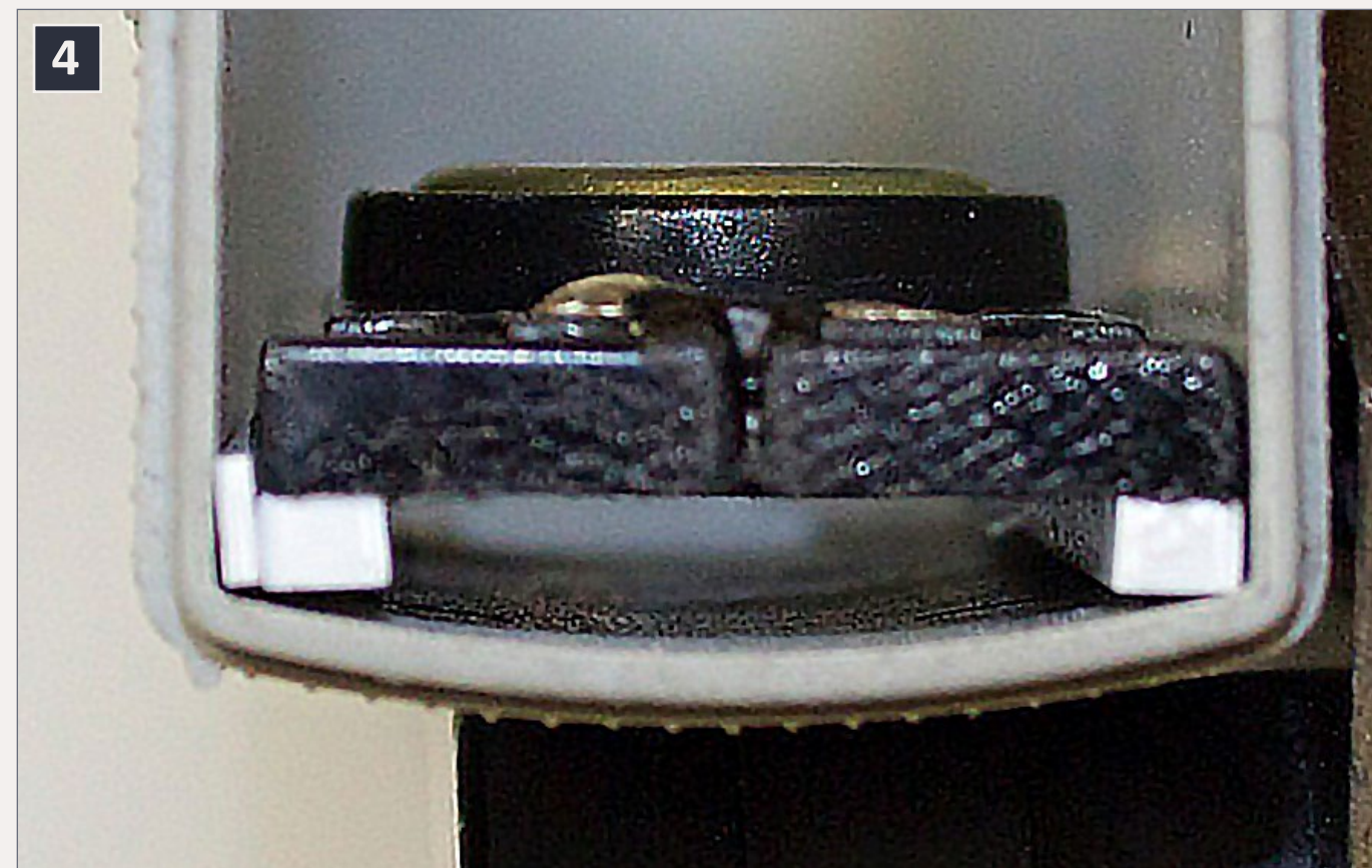
4. Speaker assembly with white plastic spacers being tested into the shell. Look below the speaker on both sides. There's a shim on the left.
