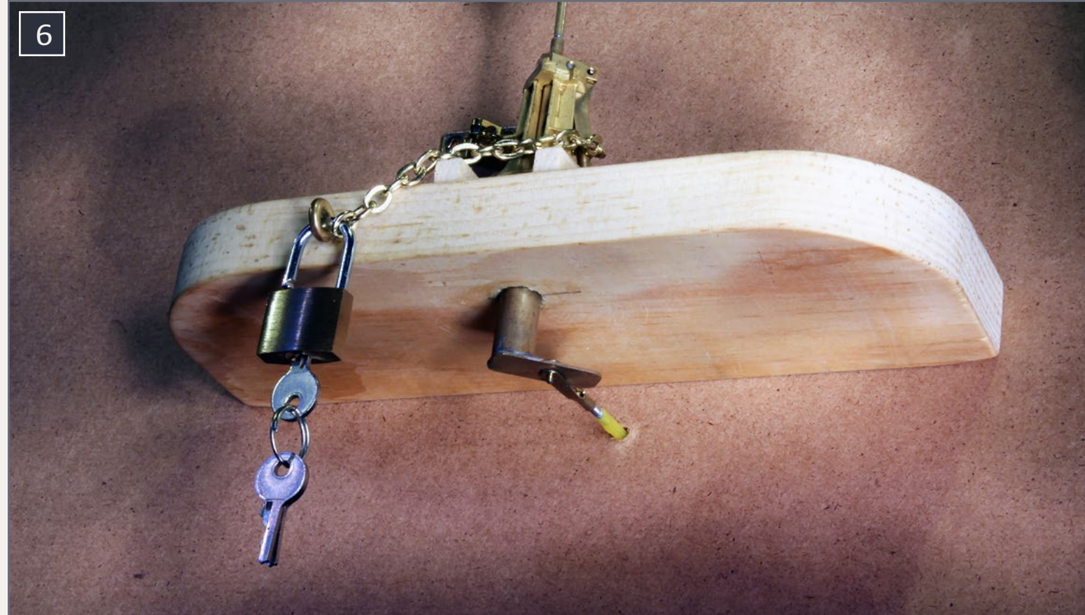
6. The modified mechanism of the switch stand projects below the shelf to connect to plastic control rods. The lock is an inexpensive luggage lock.
