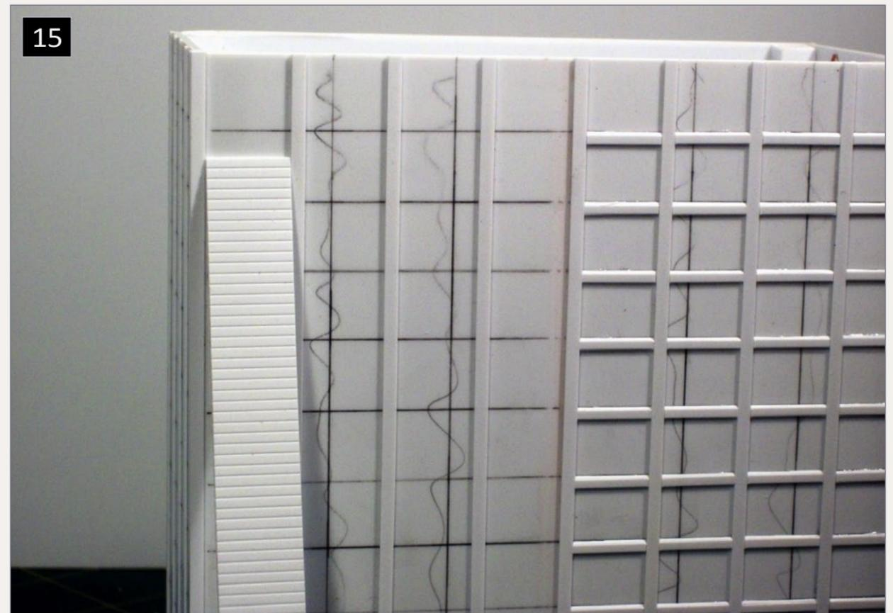
**15. In-progress photo showing the partially assembled feed bin and horizontal bracing being applied.**
