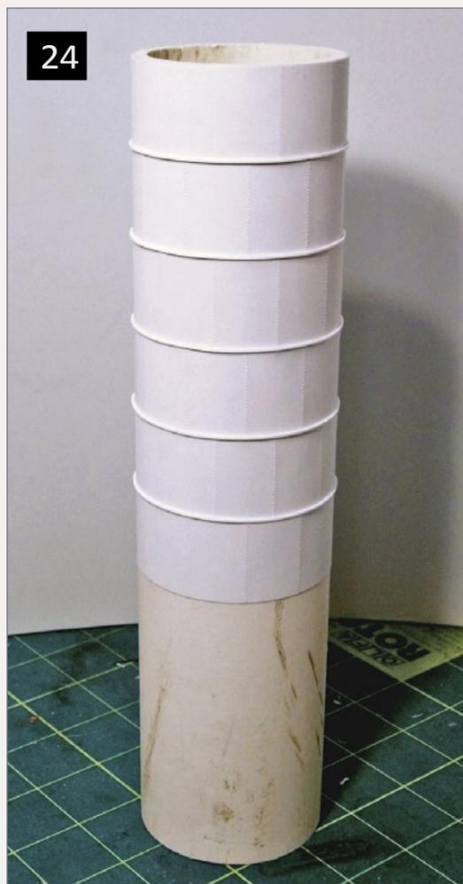
**24. In this view, the styrene panels are being applied to the end silo. The end silo construction differed than the other silos as each panel was separately wrapped with styrene. The panels were seven scale feet in height with rivets punched every five feet with overall circumference of 54.2 scale feet. Between each panel was a piece of .030" by .030" piece of styrene to match the prototype.**
