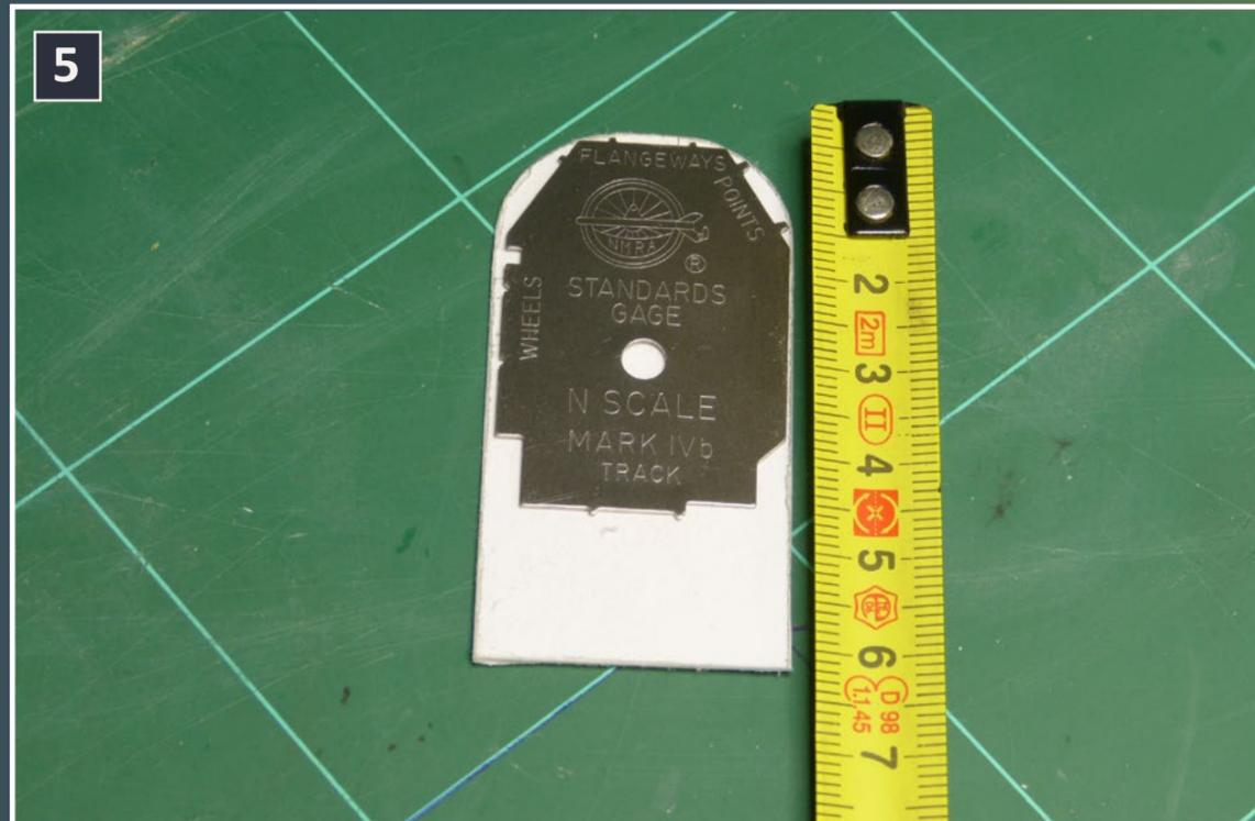
5. The arch template in comparison with a standard N scale track gauge. The top radius fits inside the profile – so motive power will fit beneath the arch.
