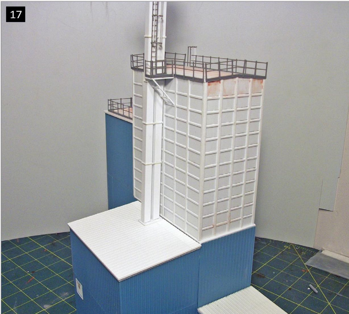
**17. View of the completed main structure with feed bin attached and elevator installed.**
