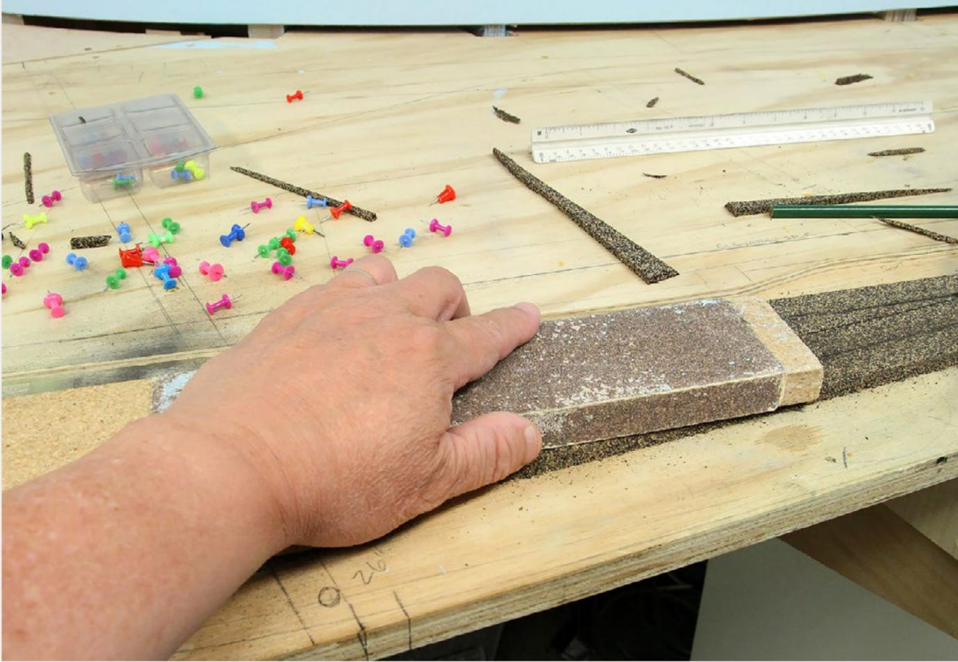
**7. Sanding gets rid of high spots and rough edges. Sanding with a long sanding block reduces side-to-side and up-and-down dipsy-doodles in the cork roadbed.**
