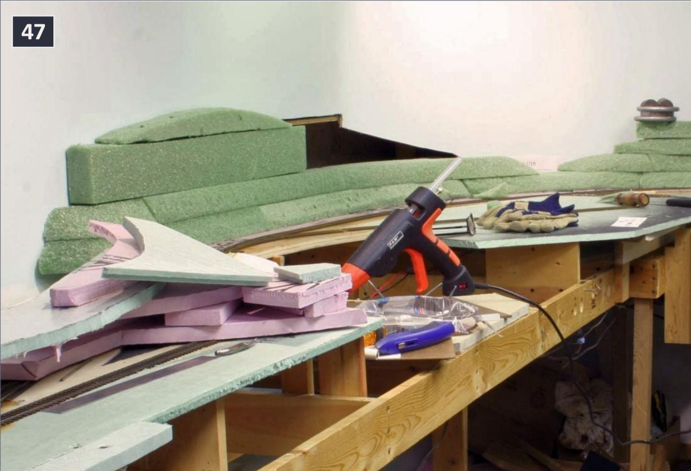
47. Here I'm beginning the second lump, the top portion of which is removable in case I need to access the track behind. The glue gun is in the future riverbed.
