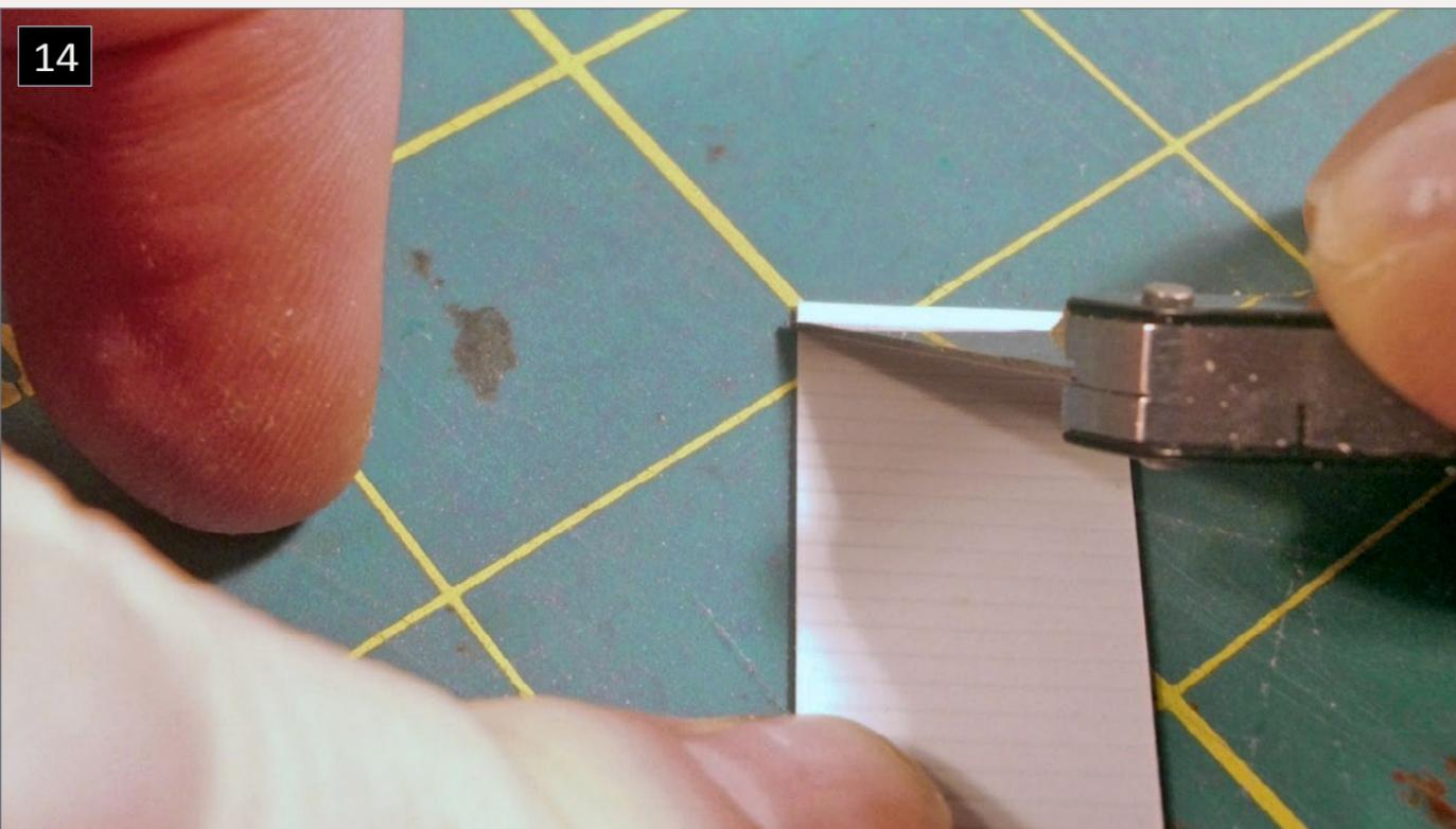
**14. Photo showing how to cut the strip styrene for the horizontal bracing on the feed bin.**
