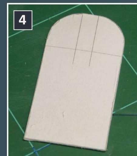
4. The final arch template. I used scissors to cut the styrene exactly along the printed line.
