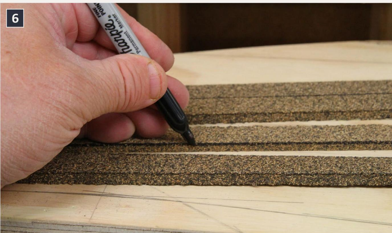
**6. Marking the edge of the cork strips before installation makes the seam where they join obvious to the casual observer. I use a black Sharpie marker.**
