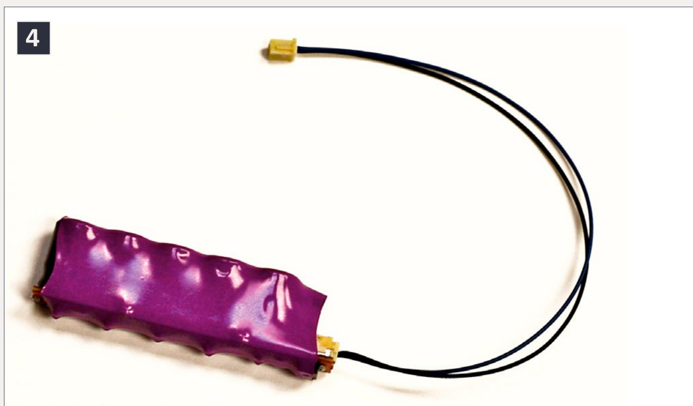
4. SoundTraxx CurrentKeeper energy storage module. SoundTraxx photo.
