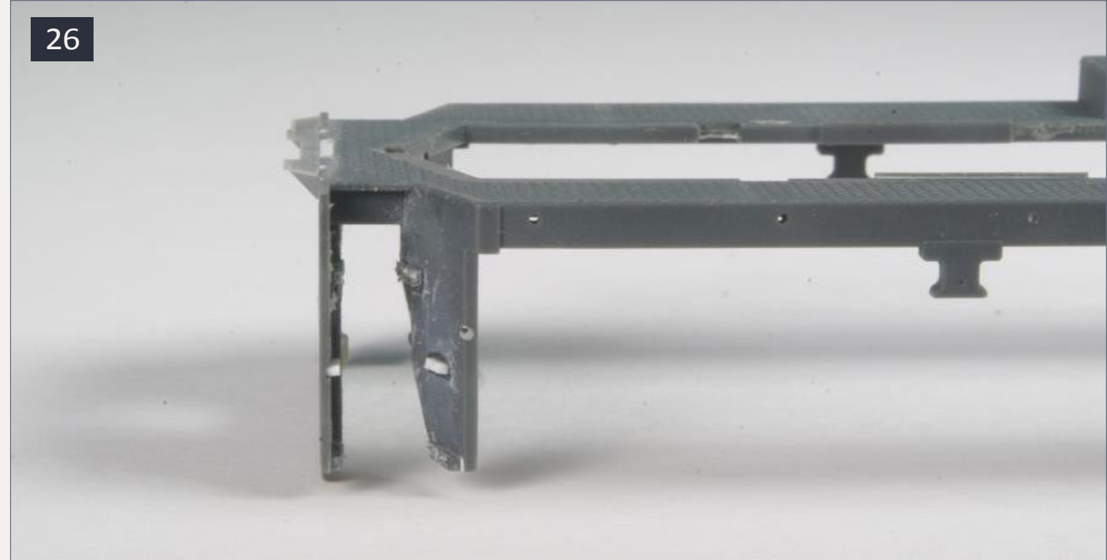
26. Sill unit with steps removed and Cannon anticlimber installed.
