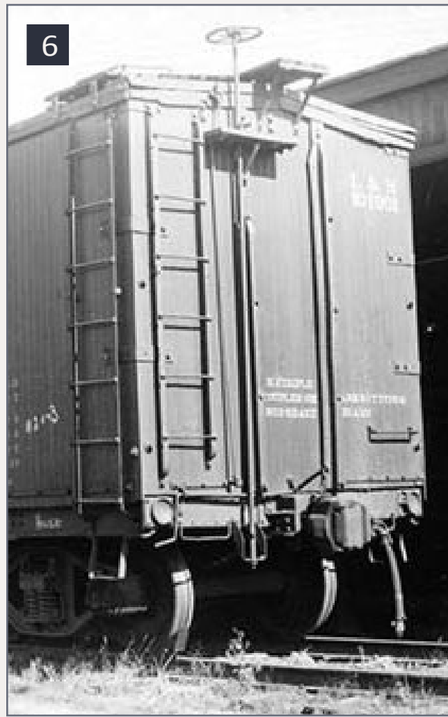
6. Double-sheathed wood car with unique vertical braces.
