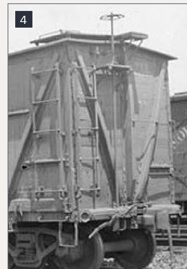
4. Distinctive 'V' braces with a single vertical brace in the center of the end.
