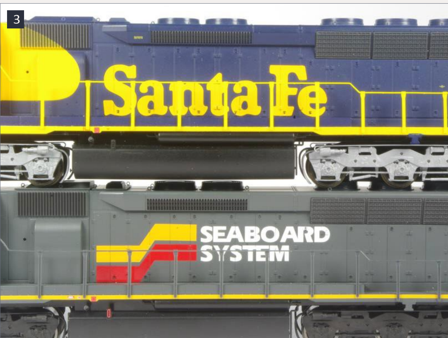
3. Comparison of the blower duct lengths on Proto 2000 SD45s.
