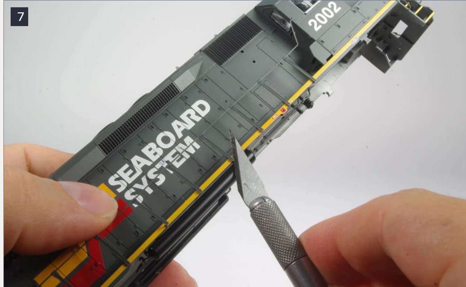
7. Removing the Proto 2000 handrails using a #11 blade.
