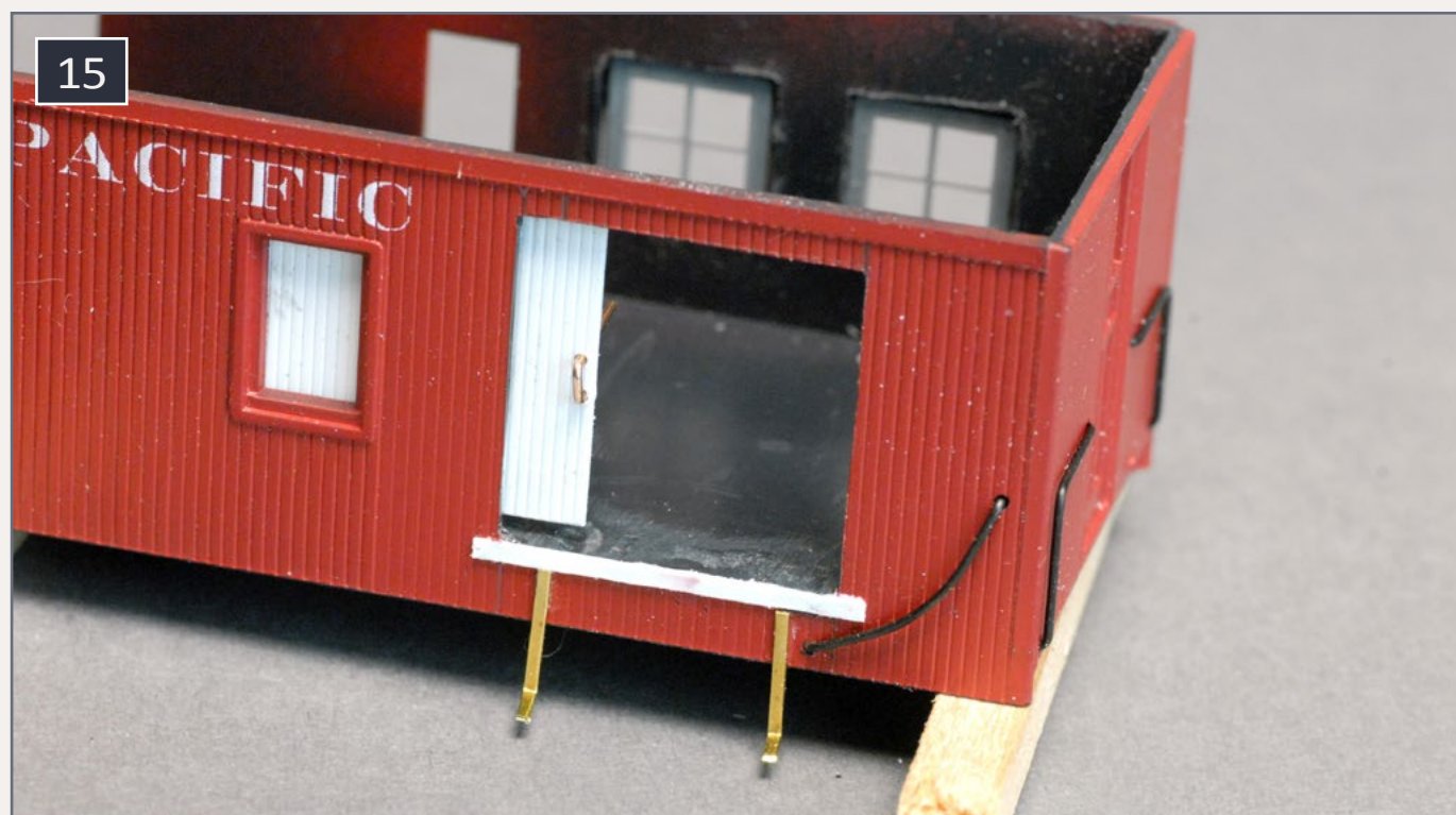
15. A cargo door was cut into the side of the caboose, and a pair of brass strip step supports were added just below the door, which later was swapped to an outside-hung version.
