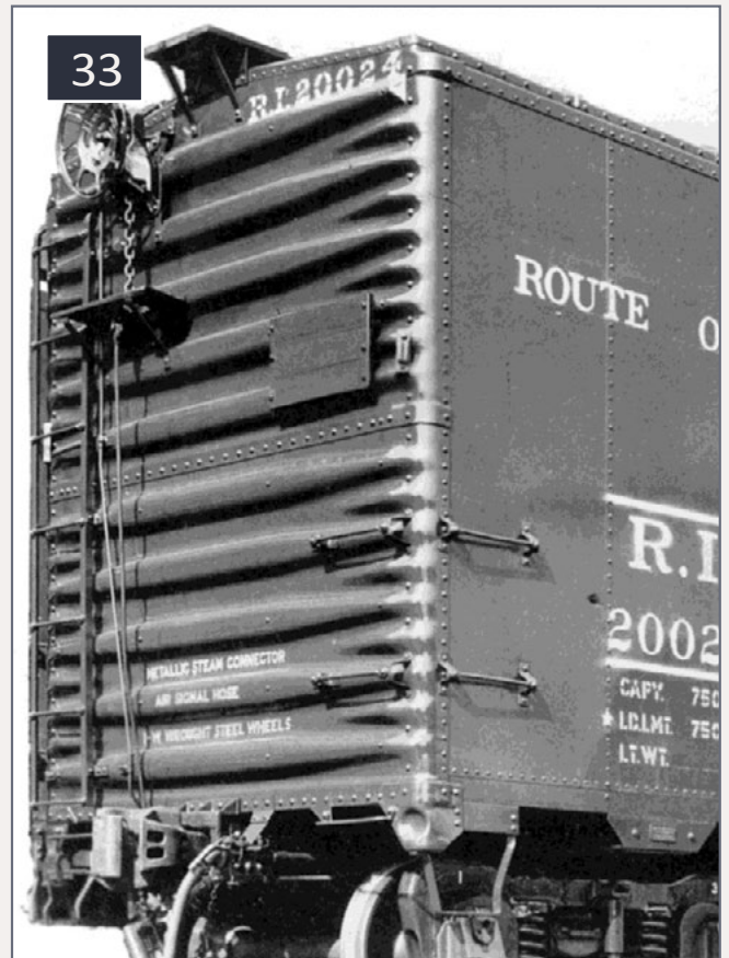
33. Dreadnaught 5/5 end with rounded corner for W-section corner post. Note truncated top rib. Car built in 1941 by Pressed Steel Corp.
