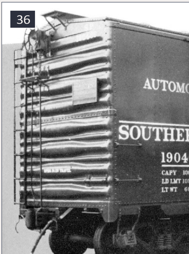
36. Improved Dreadnaught 4/4 end with main ribs shaped like rolling-pins. Note truncated top rib on this car built in 1953.
