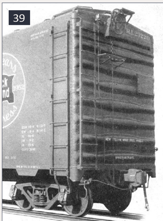
39. Introduced in the late 1930s, the dart-less end didn't gain significant favor until the late 1940s.
