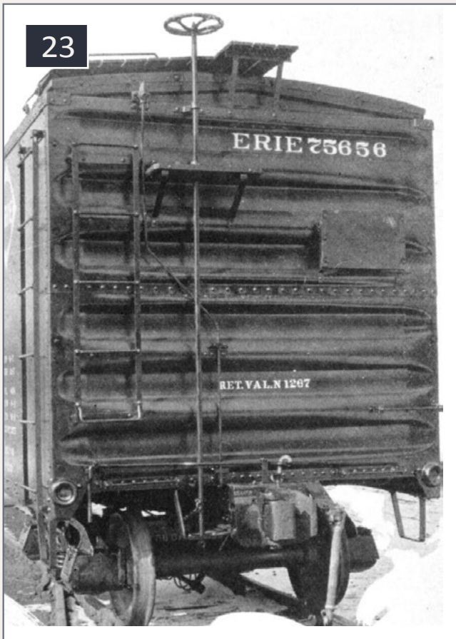
23. Buckeye two-panel end with straight corrugations that flatten at sides. Built in late 1920s by Chicago-Cleveland Car Roofing Co.
