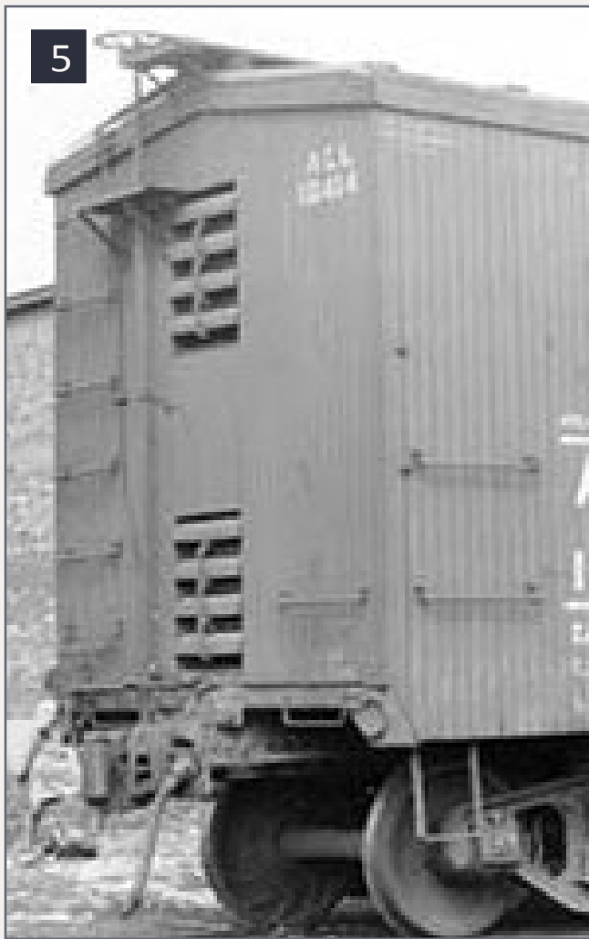
5. Double-sheathed car with vents installed between the vertical steel end braces.
