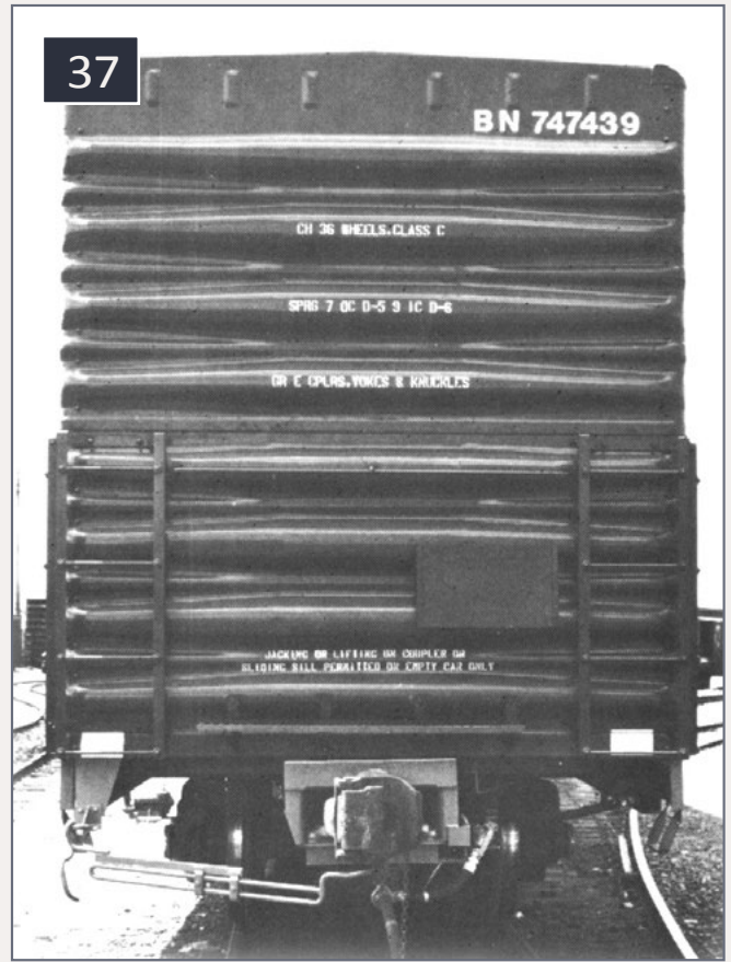
37. Improved Dreadnaught end on car built by Pacific Car & Foundry. Note non-tapered top rib and six small vertical indentations in the hat section.
