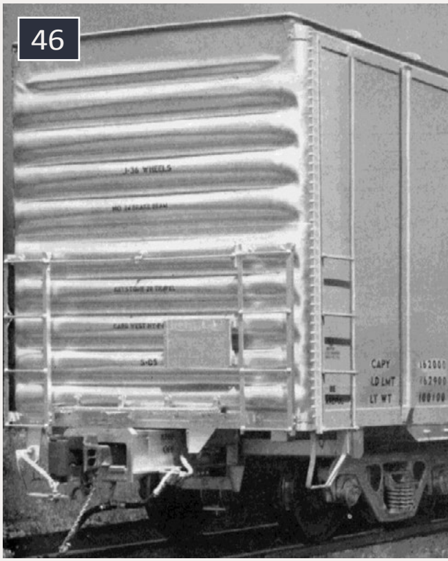
46. P-S-built this car in the late 1960s using 4/5 ends with bold nontapering ribs. Note the small short rib at the top.
