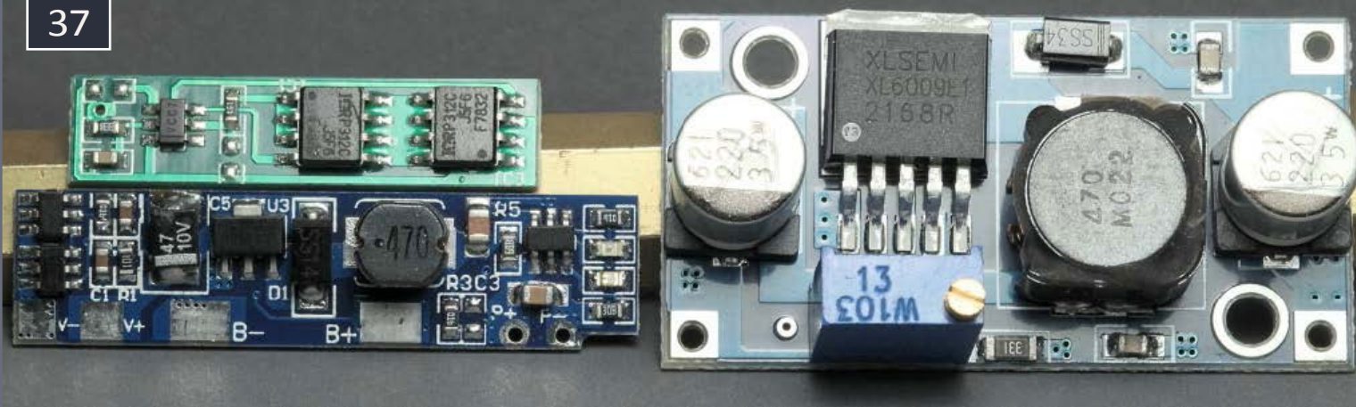
37. Battery manager (on left) and DC-DC converter.
