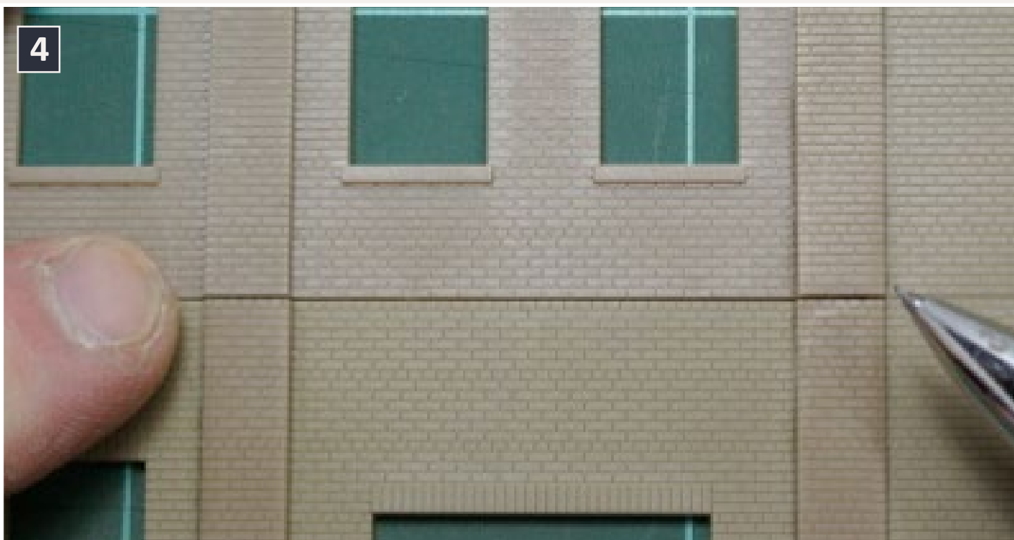
4. Precision sanding and filling might hide the gap between modular sections, but would also take a lot of time.
