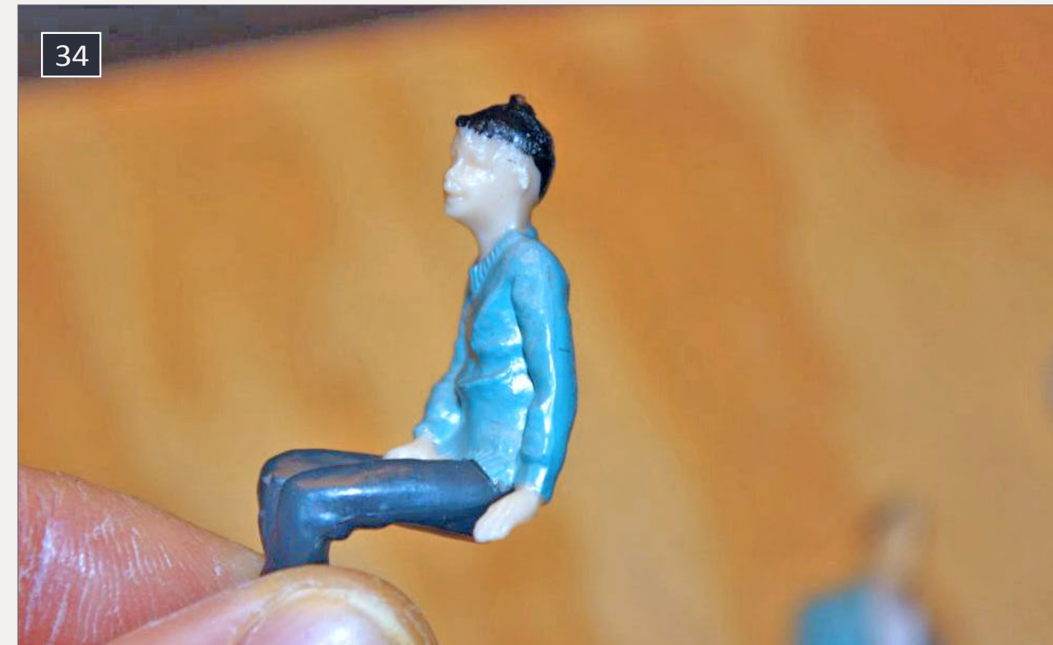
34. Figure has molding flash to be removed
