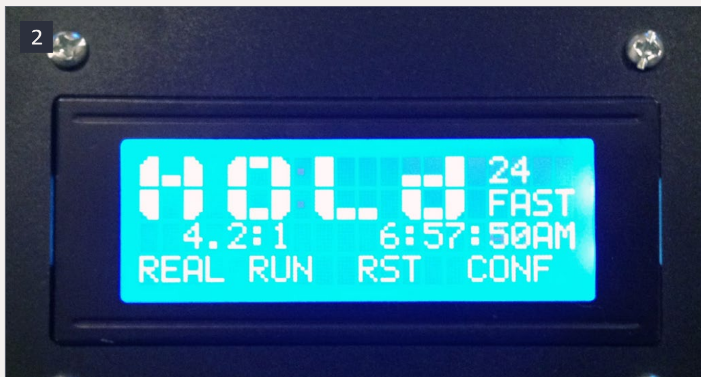
2. Master clock in Hold mode, also showing my chosen fast clock ratio of 4.2/1.
