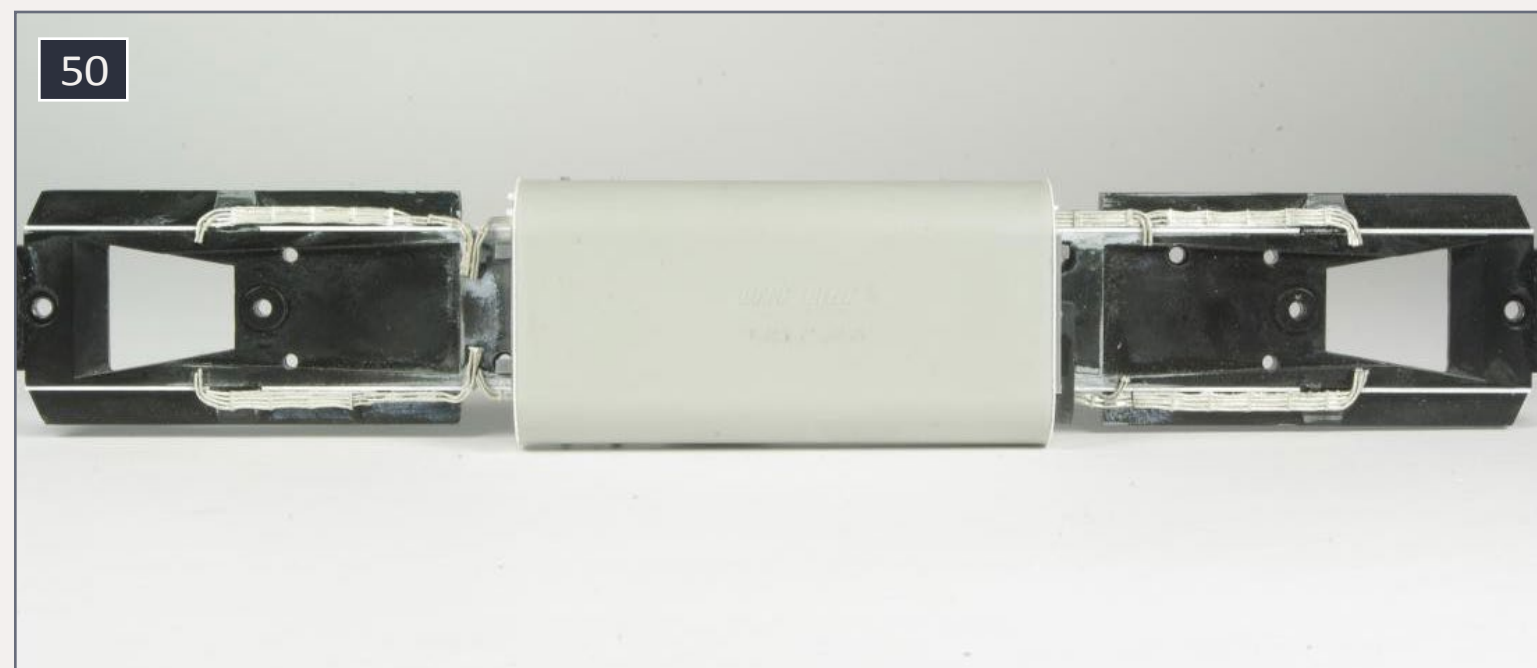
50. Bottom view showing traction motor cable routing.
