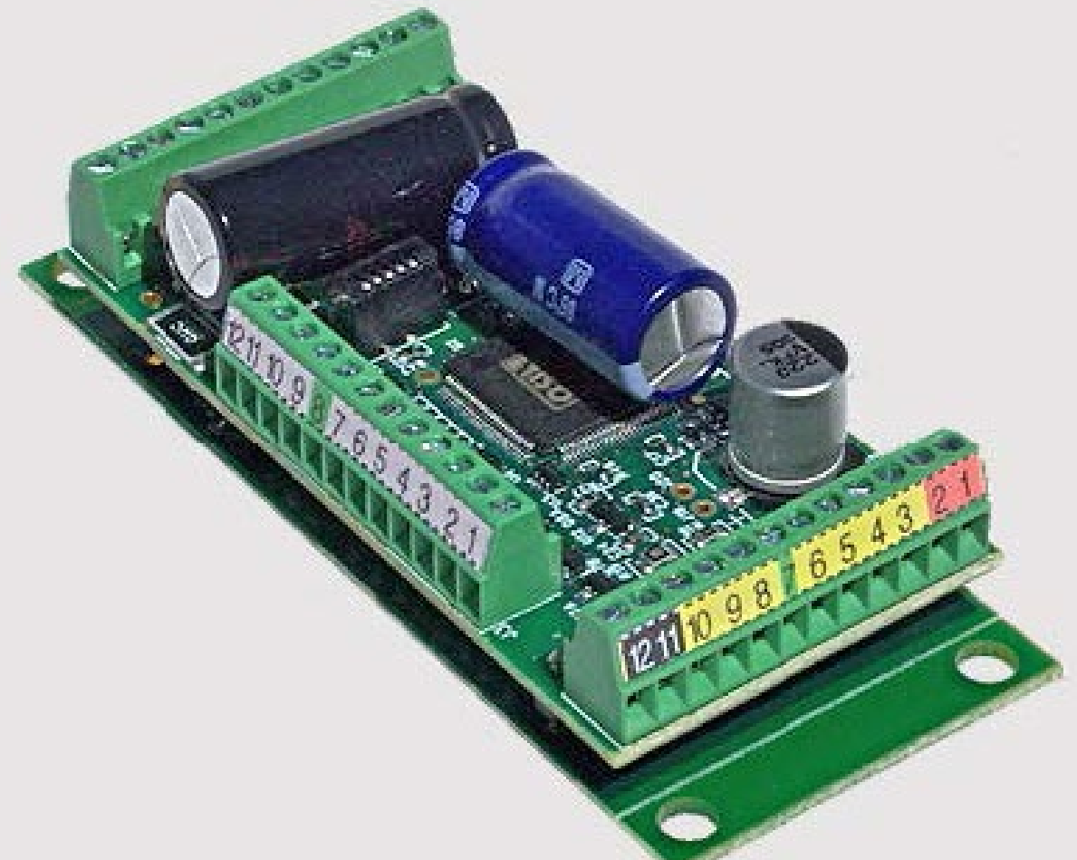
8. QSI Titan Magnum decoder rated for 6-amp stall, 10-amp run. QSI photo.
