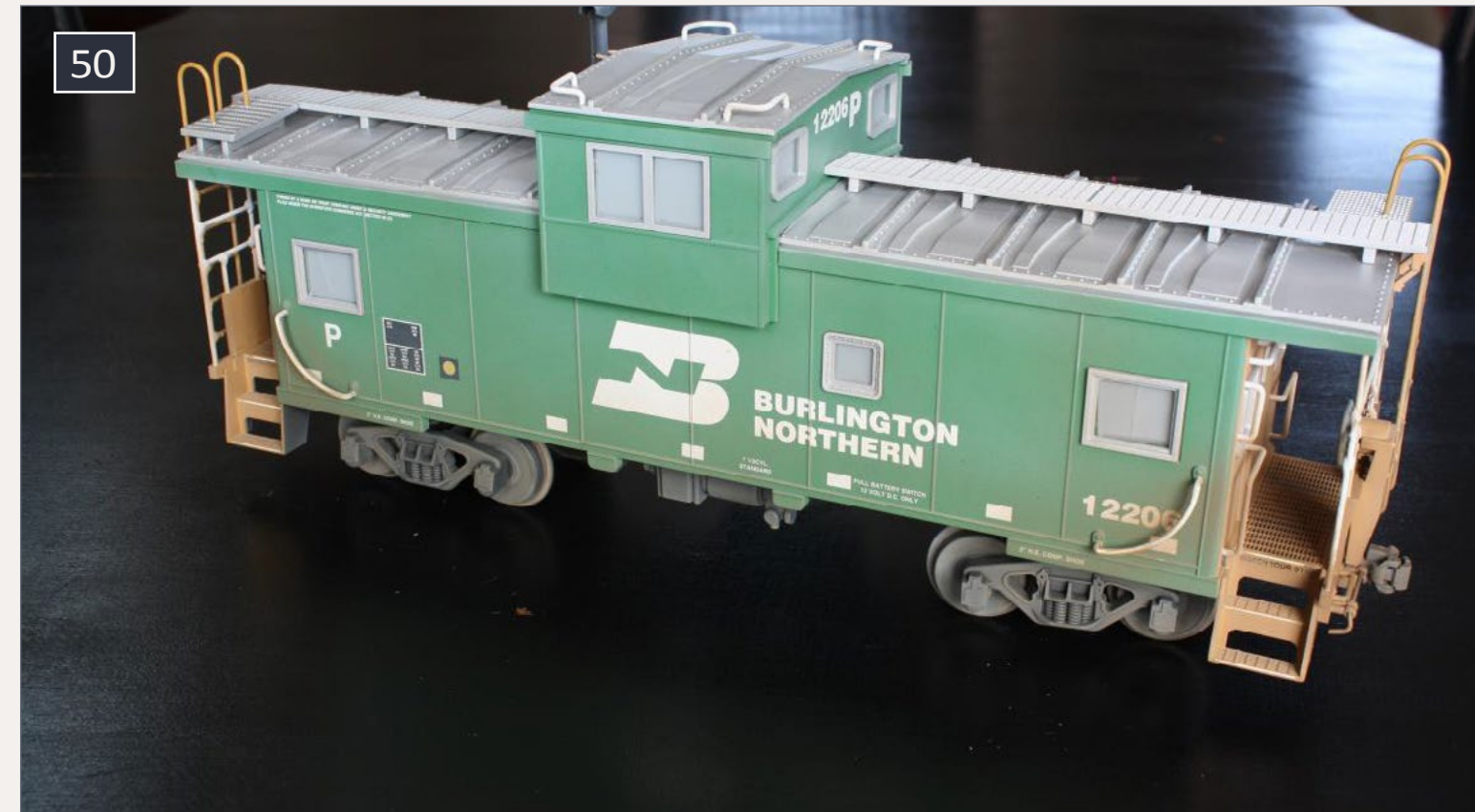
50. Light gray wash and dirt color have been airbrushed.
