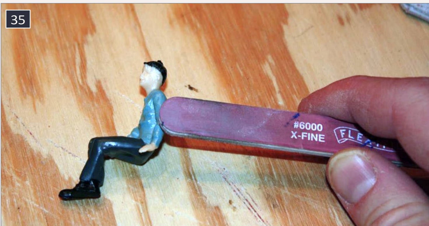
35. Using a sanding stick to remove molding lines on arms and legs.
