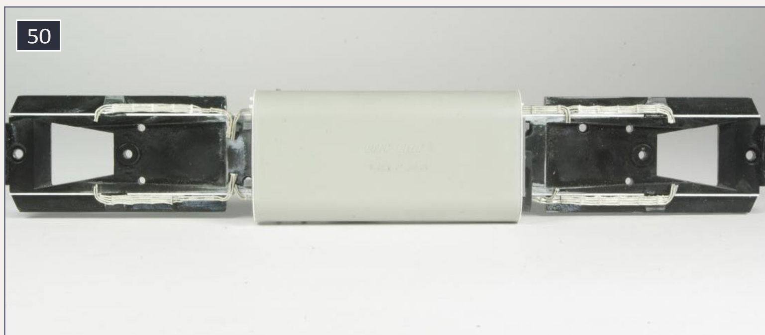
50. Bottom view showing traction motor cable routing.
