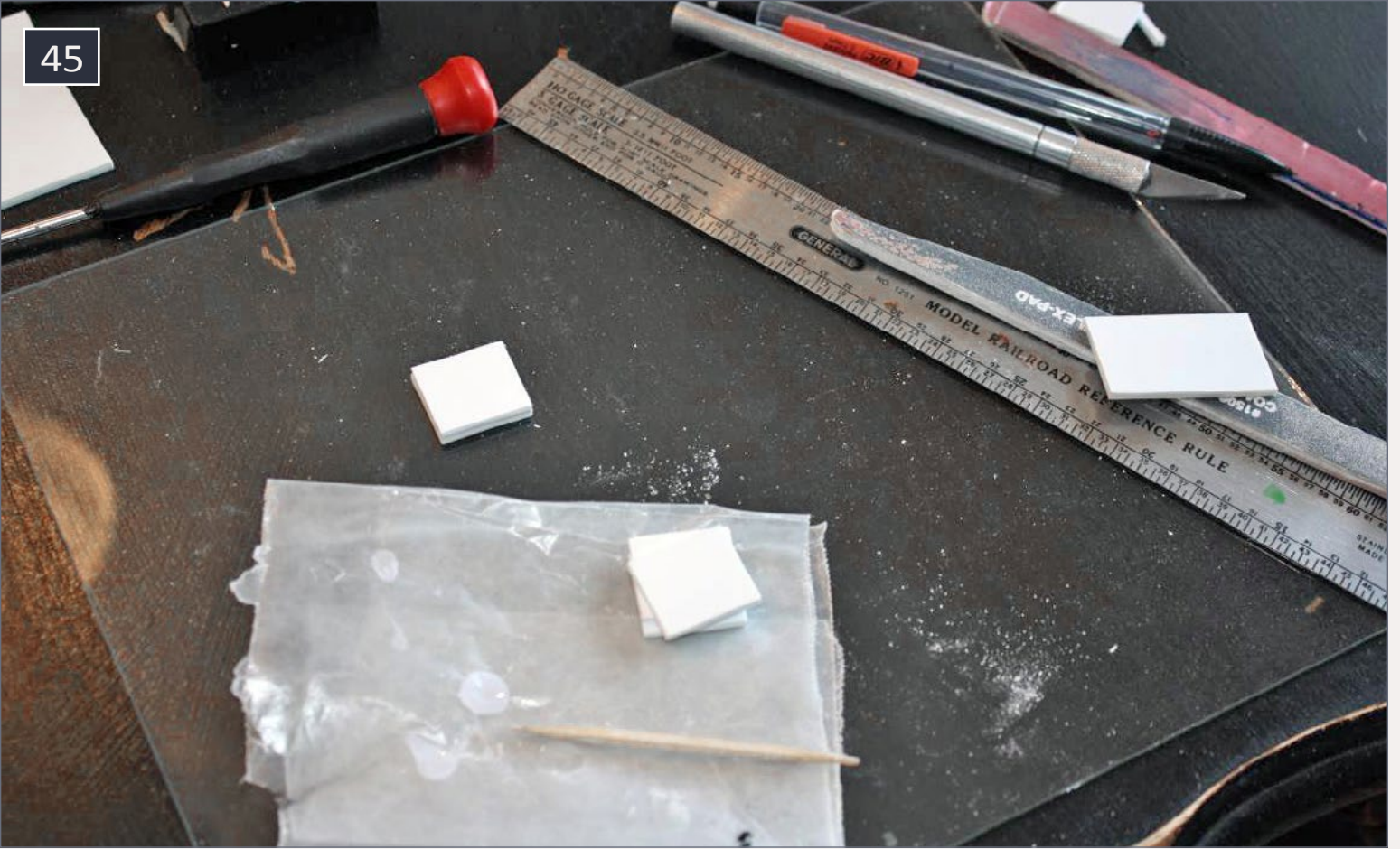
45. Building the coupler mounting box from styrene.
