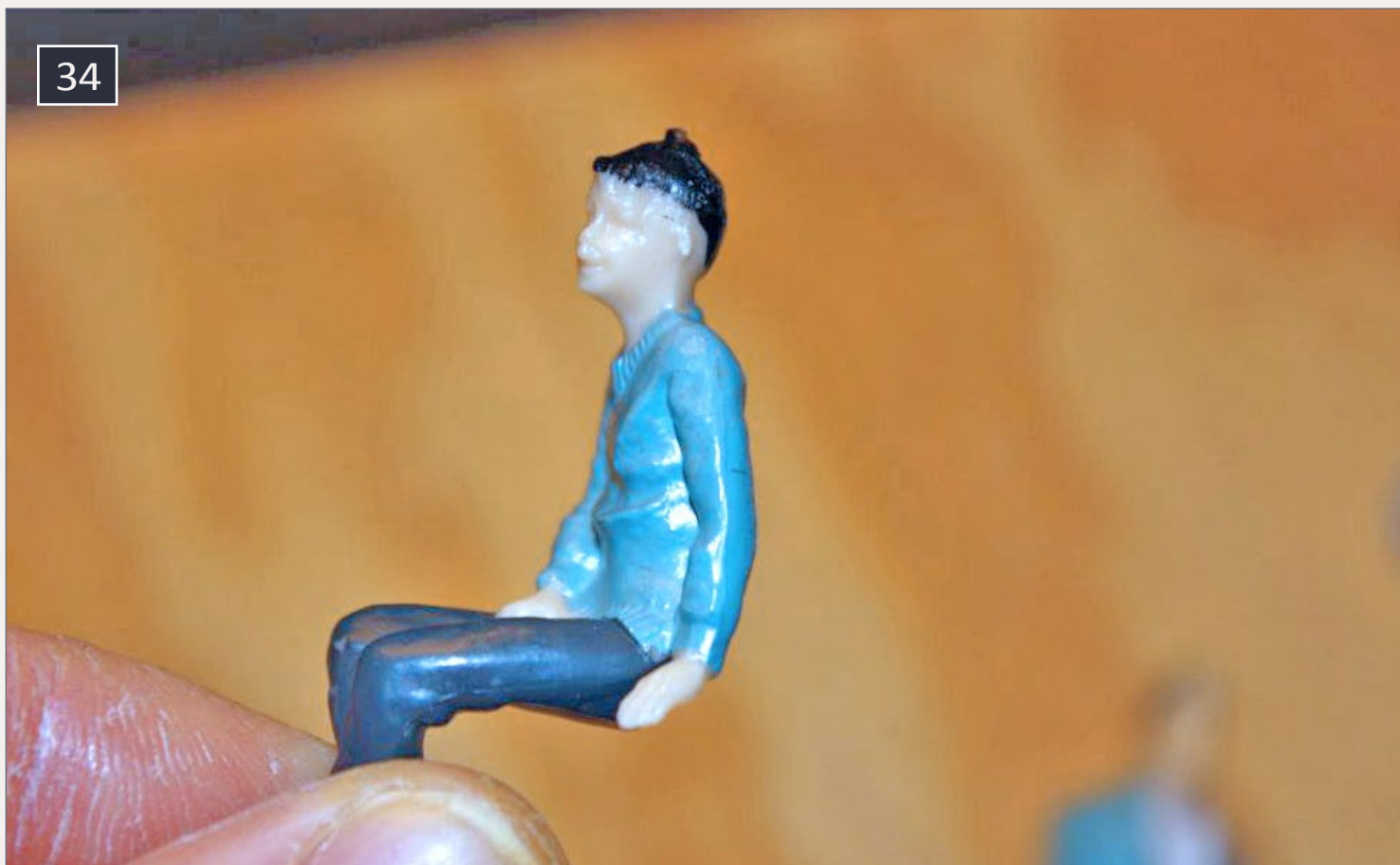
34. Figure has molding flash to be removed
