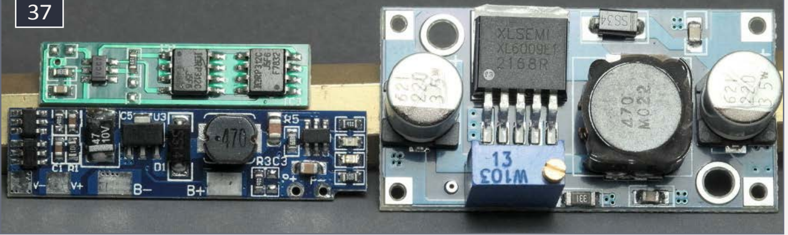
37. Battery manager (on left) and DC-DC converter.
