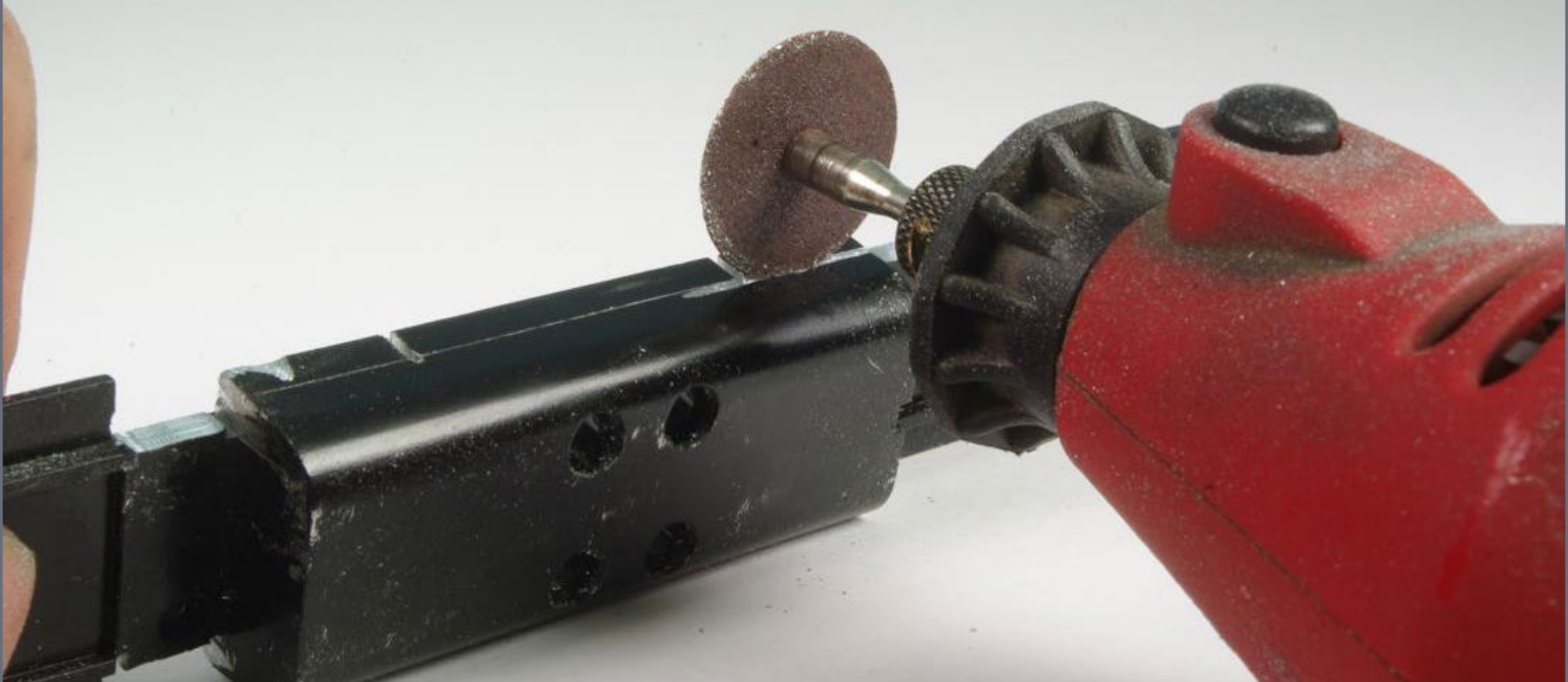
42. Making the horizontal cut to the fuel tank.
