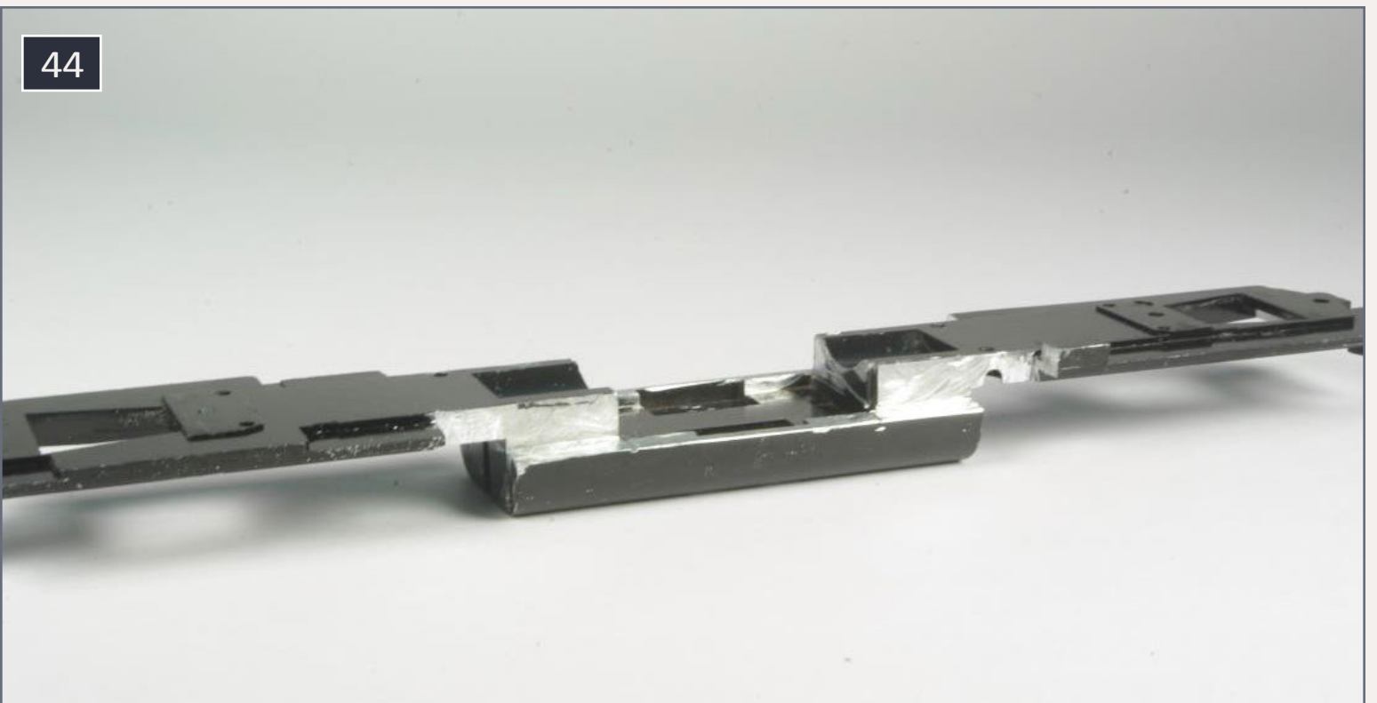
44. The frame after all cuts and milling.
