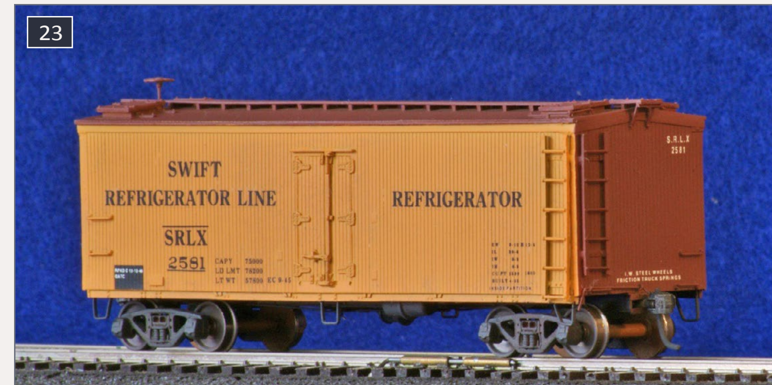
23. The finished car, decaled and over-sprayed with Dullcote
