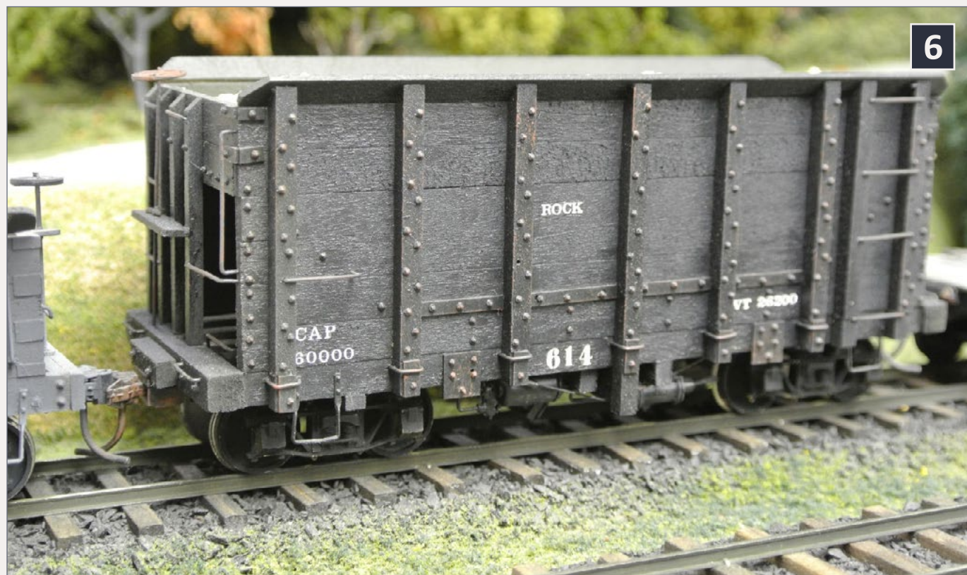
6. On3 model of Hancock and Calumet car in service on David Crement's East Broad Top layout. The car is scratchbuilt. This is an updated car with steel lining and Vulcan trucks. David Crement photo.
