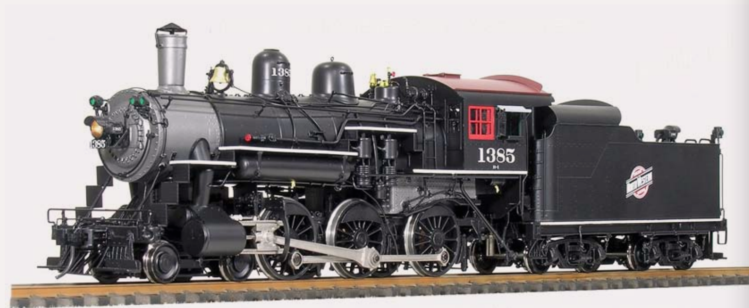
FIGURE 15: This O scale model is a preproduction sample of a C&NW 4-6-0 class R-1 under development by brass importer Glacier Park. Four distinctly different versions of the R-1s (numbers 50, 487, 1385 and 1400) will be created in order to provide an historically accurate cross section of the life of the reliable steamer. The models are being handcrafted in Korea by Boo-Rim Precision. A Proto-48 conversion kit will also be available. www.glacierparkmodels.com .
