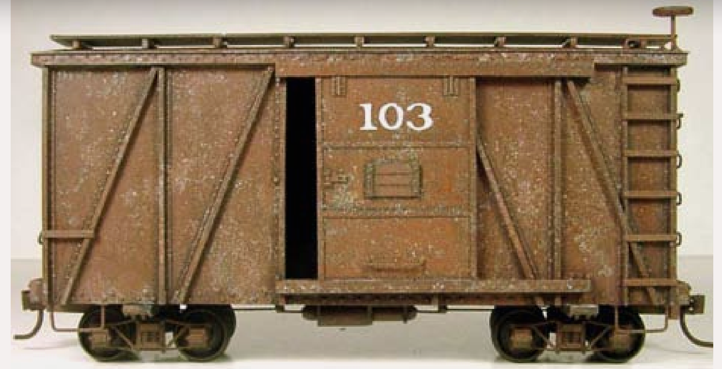
FIGURE 9: This funky On30 narrow gauge 20-foot steel boxcar was assembled from a kit available now from Boulder Valley Models. All of the details shown are included except trucks and couplers which are sold separately. See www.bouldervalleymodels.com
