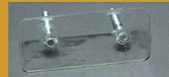
Figure 2: The plastic base for the cleaning pad with threaded rods flush with the sheet.
