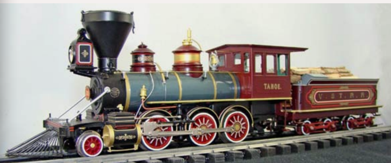
Figure 16: Pilot model of V&T Mogul uses 3-rail type wheels with the typical oversized flanges. The 2-rail models have standard R-25 wheel flanges.
