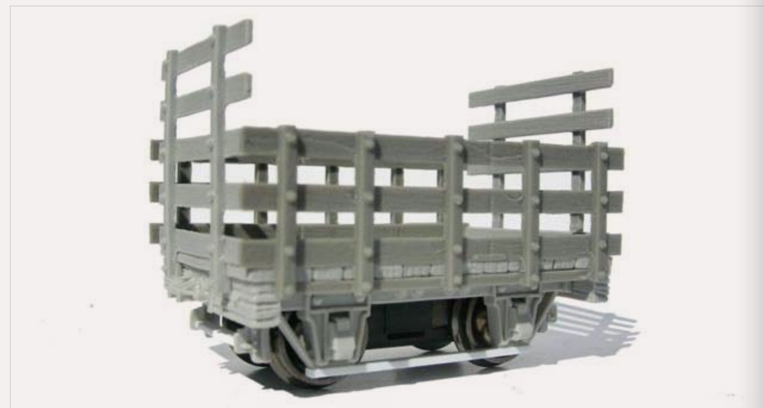
FIGURE 1: Here is a preview look at a unique On30 scale powered car under development by Backwoods Miniatures ( www.backwoodsminiatures.com ) . The cast resin body is mounted on a Tenshodo SPUD power unit. Delivery date and pricing are pending.
