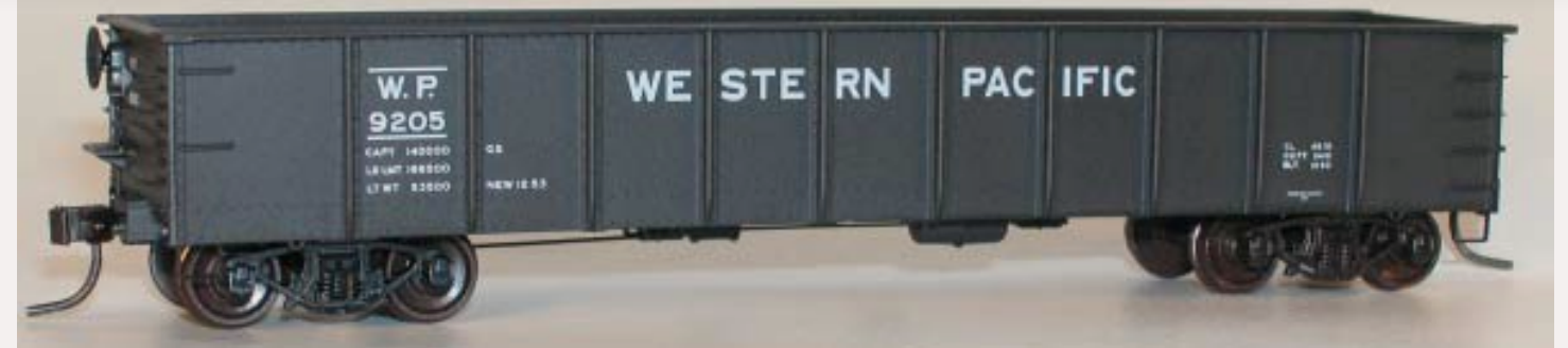
FIGURE 3: Digital Fox ( www.digitalfox.com ) is offering this ready-to-operate Western Pacific 41-foot steel gondola based on an Accurail model. The HO scale car comes with Accumate magnetic couplers and Delrin wheelsets. Visit www.digitalfox.com for details.
